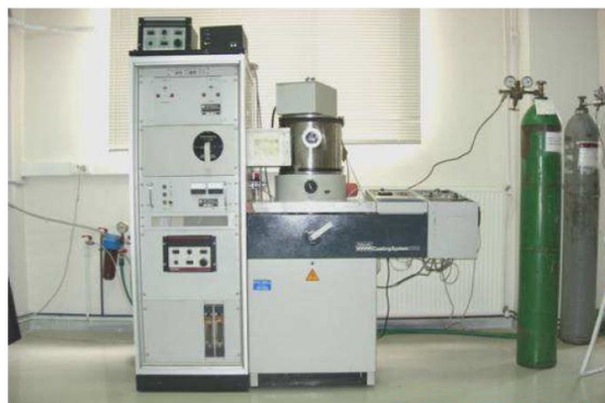
Figure 3.1: Photo of the Edwards 306A sputtering unit installed at INN, NCSR ‘Demokritos’.
