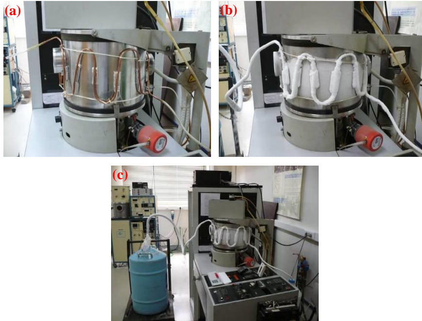
Figure 3.3: Photos of a magnetron sputtering equipped with the homemade cryotrap obtained (a) before and (b),(c) during the cooling procedure.
