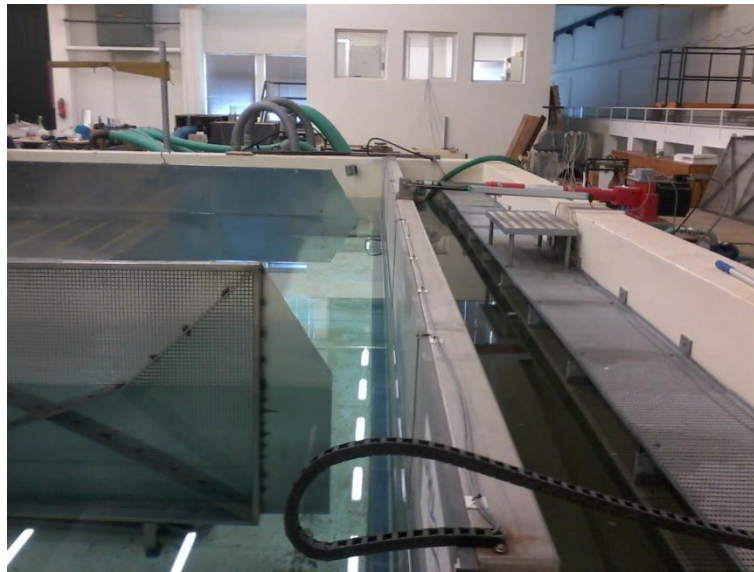
Fig. 5.11. Side view of the wave maker and the electric actuator.
