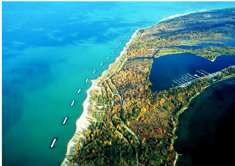
Fig. 7.1. (a) Tombolo behind a system of emergent breakwaters in Norfolk, England, 2015 (photo: Jonathan Webb) and (b) salient behind an array of emergent breakwaters in Presque Isle, Pennsylvania, U.S.A. (from Mohr, 1994).
