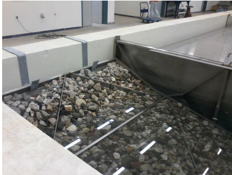
Fig. 5.9. View of the absorbing layer at the down-wave boundary of the wave tank.
