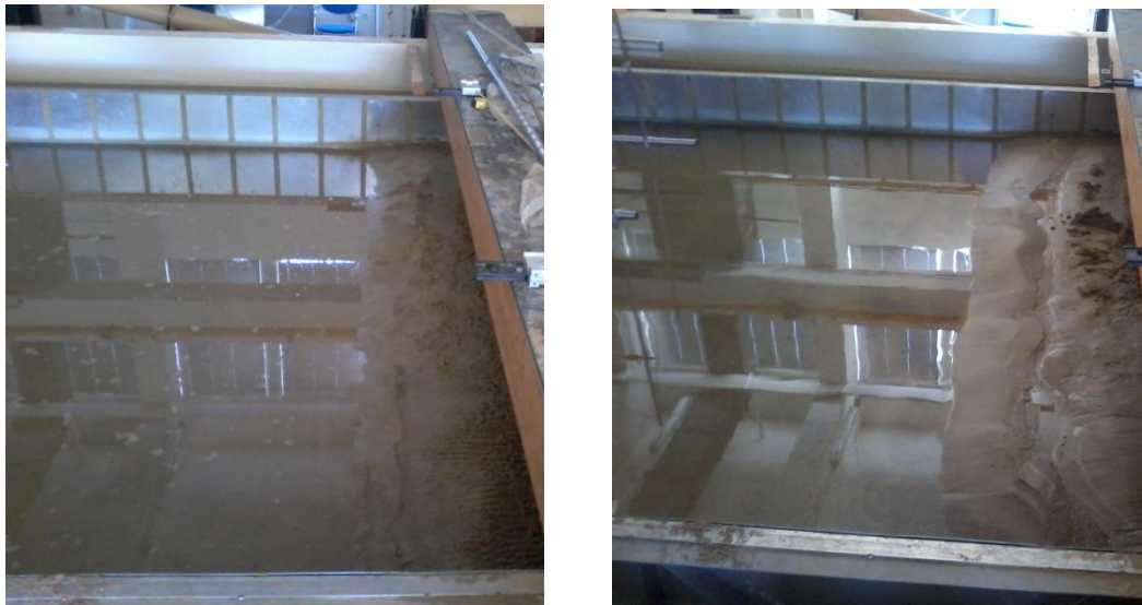
Fig. 6.15. View of the initial (at left) and final (after 4 hrs of wave action, at right) shoreline for test case 1.
