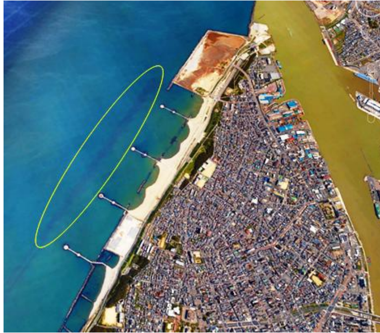
Fig. 1.4. Aerial view of a submerged breakwater (in yellow ellipse) in Niigata beach, Japan (from Google, 2016).
