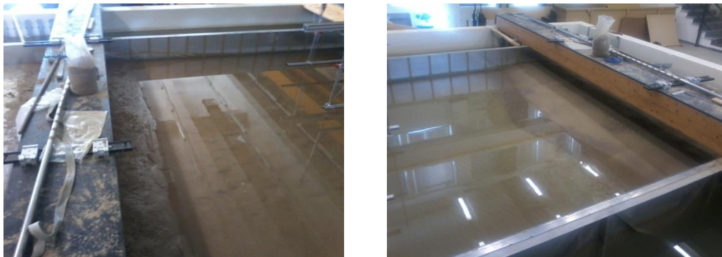
Fig. 6.57. View of the initial (at left) and final (after 5 hrs of wave action, at right) shoreline for test case 7.
