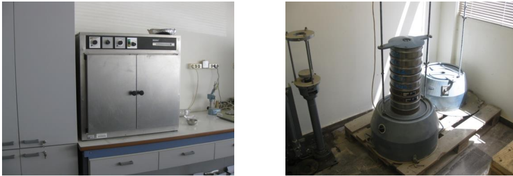
Fig. 5.15. Oven for drying the sediment samples (at left) and sieve vibrator (at right).
