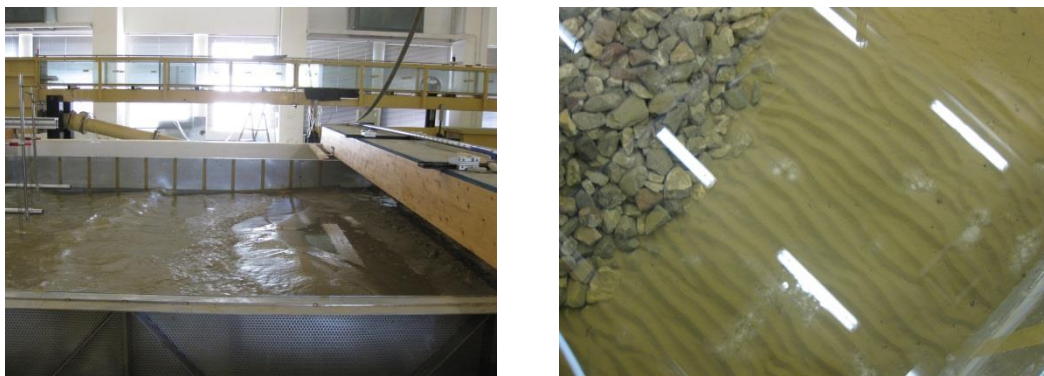
Fig. 5.17. Snapshot of wave propagation (at left) and bed wave ripples close to the gap (at right).
