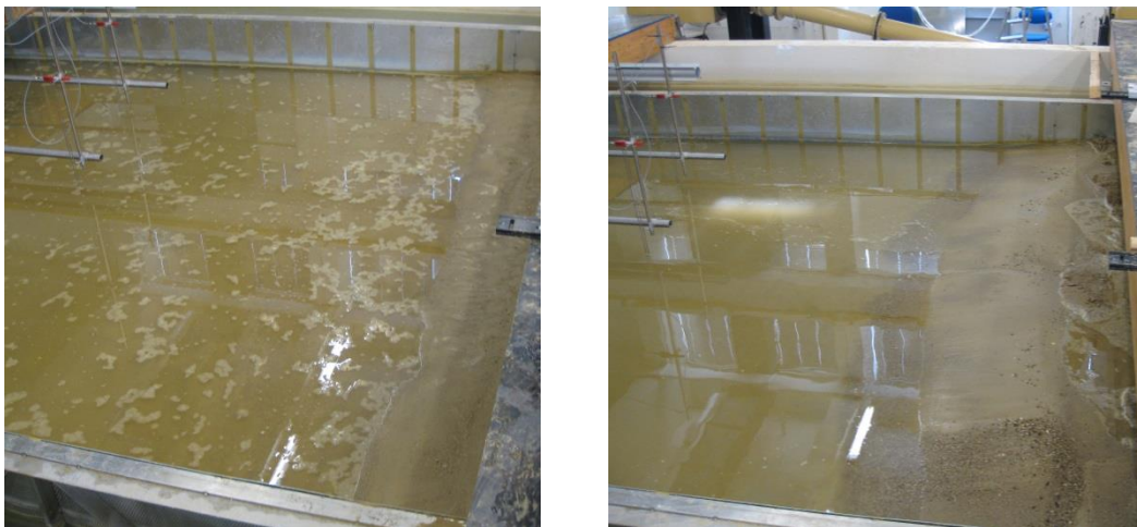
Fig. 6.33. View of the initial (at left) and final (after 4.3 hrs of wave action, at right) shoreline for test case 4.
