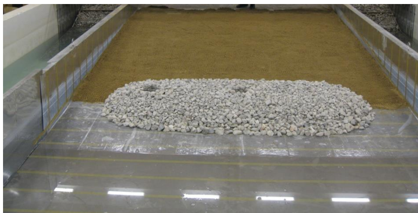
Fig. 5.14. View of the submerged breakwater and the sandy beach.
