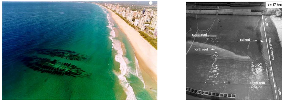
Fig. 5.1. Aerial view of the V-shaped artificial reef at the Gold Coast, Australia (at left) and the corresponding physical model at the Water Research Laboratory of University of New South Wales, Australia (at right, from Ranasinghe and Turner, 2006).
