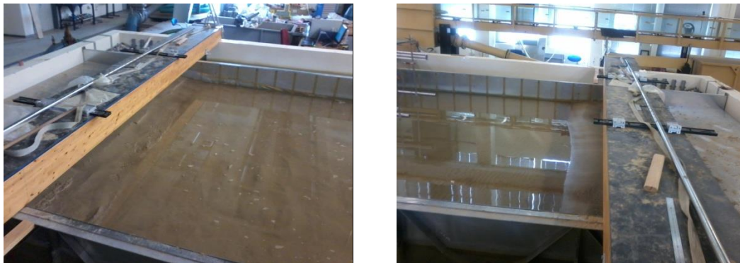
Fig. 6.43. View of the initial (at left) and final (after 5 hrs of wave action, at right) shoreline for test case 5.
