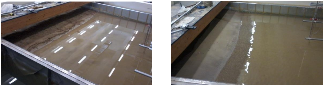
Fig. 6.64. View of the initial (at left) and final (after 5 hrs of wave action, at right) shoreline for test case 8.
