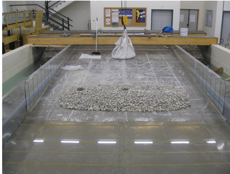
Fig. 5.13. View of the submerged breakwater.
