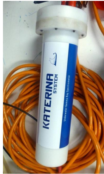
Fig. 2.23: The underwater detection system KATERINA (Tsab_08).
