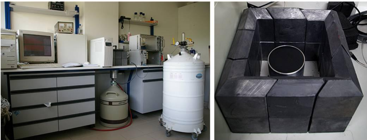
Fig. 2.25: The HPGe detector (left) and the Pb shielding (right) at the facilities of the HCMR.
