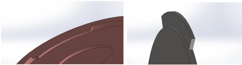
Figure 15 . View of the cavities in which the blades (next) are being inserted
