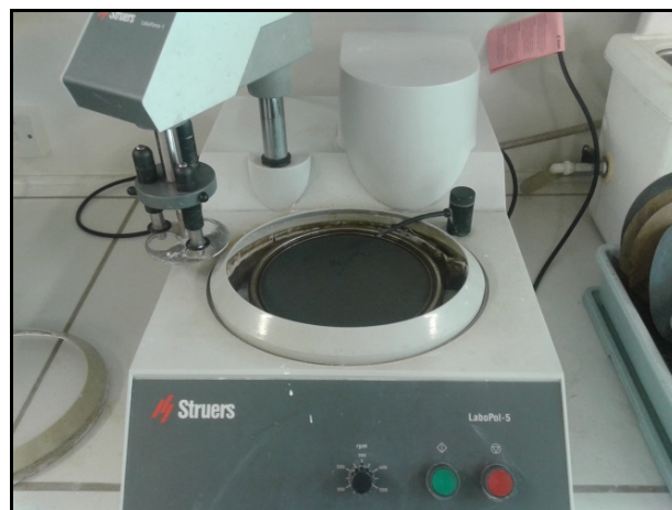
Figure 3.9: Machine of abrasion / polishing Struers LaboPol-5 the Lab. of Naval Technology
