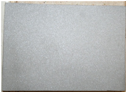
The sandblasted surface
