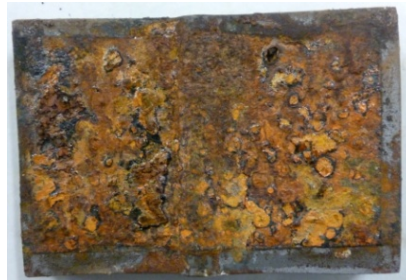
The corroded surface
