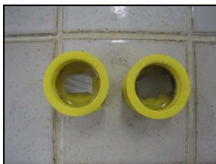
Figure 3.8: Specimens immersed with an epoxy resin
