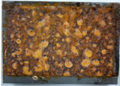
The corroded surface
