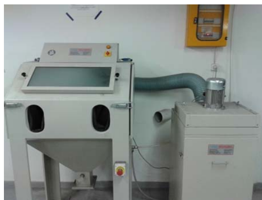
Figure 3.16: Sandblasting machine of the Laboratory of Naval Technology
