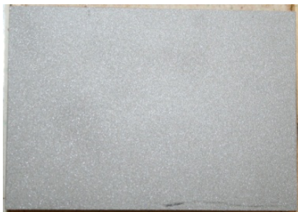
The sandblasted surface
