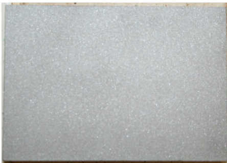
The sandblasted surface
