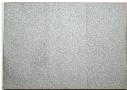
The sandblasted surface
