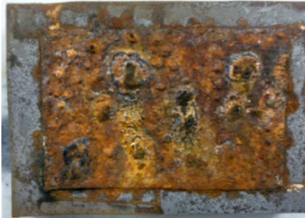
The corroded surface
