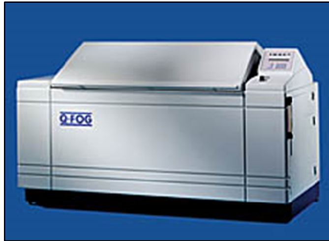
Figure 3.14: Salt Spray Chamber (Q FOG CCT 1100)
