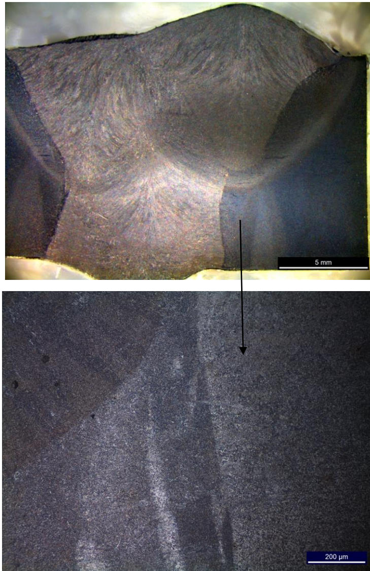
Figure 4.8: Heat affected zone in the 1 st pass.
