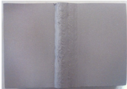
The sandblasted surface
