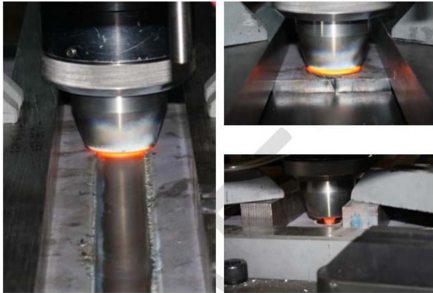
Figure 3.7: A weld being made in AH36 steel at a tool traverse rate of 100mm/min. This weld was witnessed by a surveyor from Lloyd's Register.
