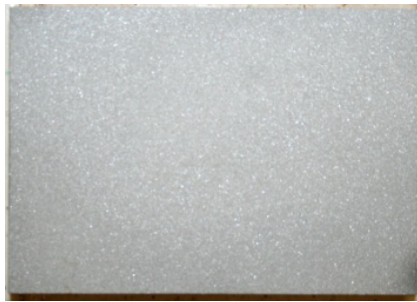
The sandblasted surface
