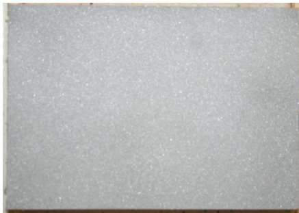
The sandblasted surface
