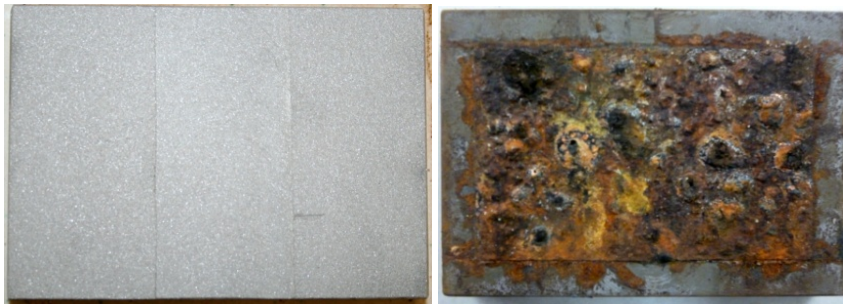
The sandblasted surface
