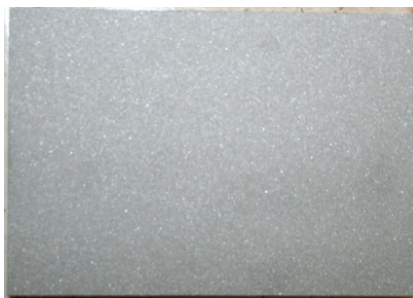
The sandblasted surface
