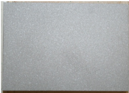
The sandblasted surface
