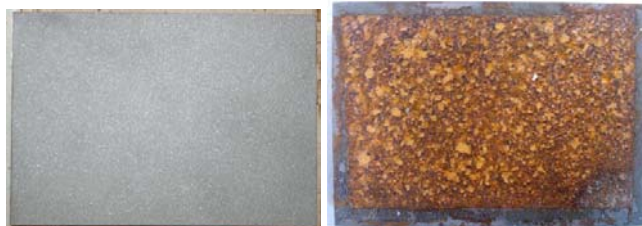
The sandblasted surface The corroded surface
