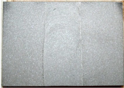
The sandblasted surface
