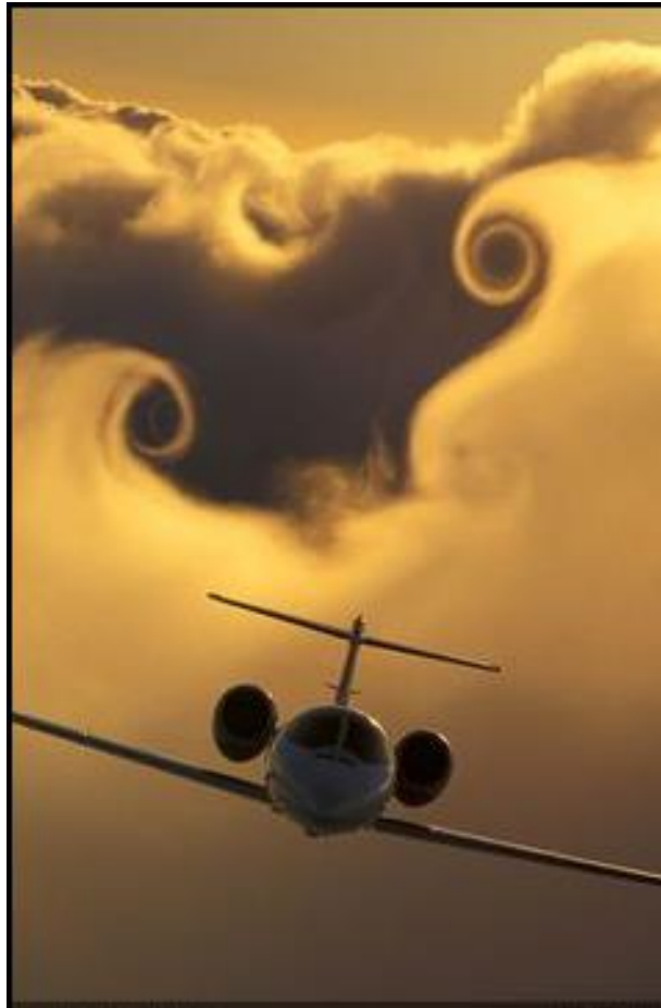
Figure 40 Wing tip vortices from a flying plane
