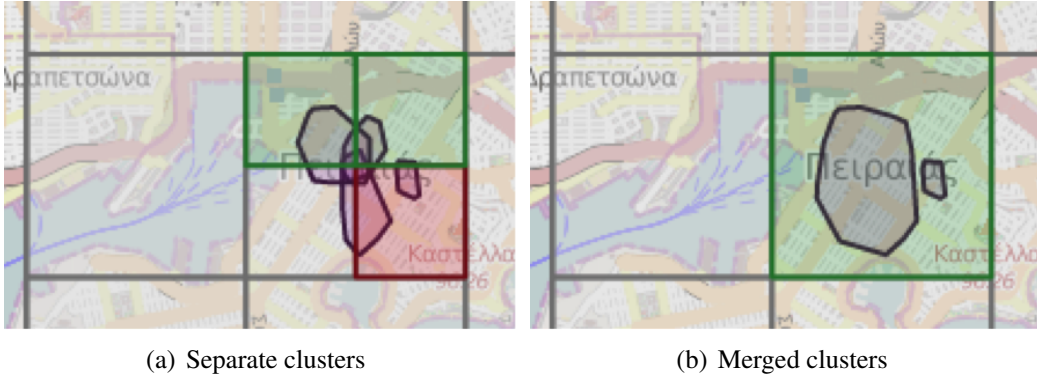
Figure 4.3: Independently calculate regions of interest for leaf nodes, then merge them into a single cluster.
