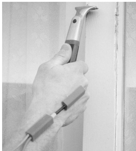
Figure 17: Example of wrist posture measurement with an electrogoniometer
