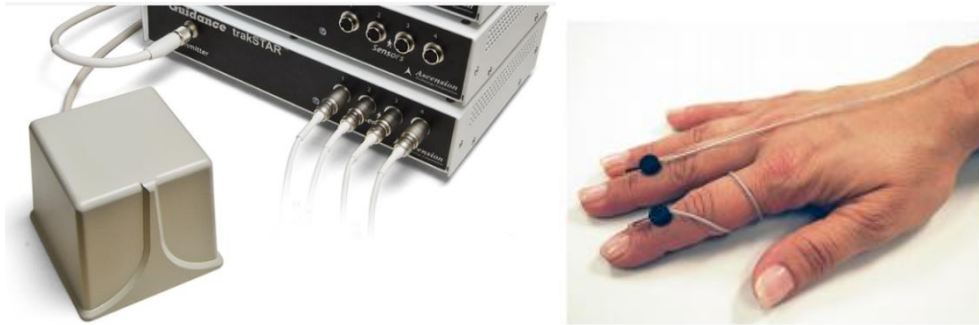
Figure 25: Example of Electromagnetic Tracking. External transmitter & finger-mounted receivers
