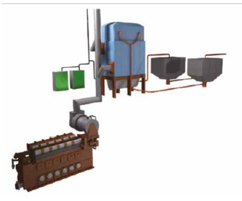
Figure 13 Couple Systems dry SO x scrubber for marine use (image courtesy of Couple Systems)
