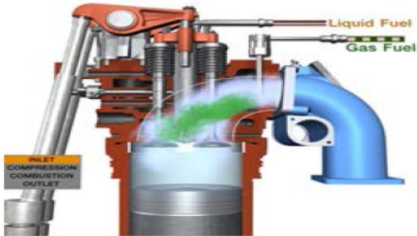
Figure 26: Wartsila duel-fuel (DF) engines_(Source Wartsilla)
