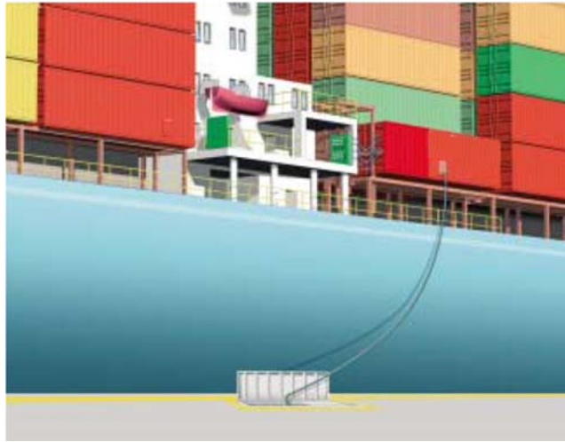
Figure 5-6 - Mobile ship-based cable management system
