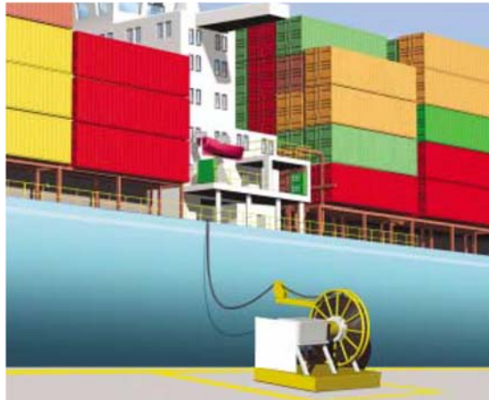
Figure 5-3 – Fixed shore-based cable management system
