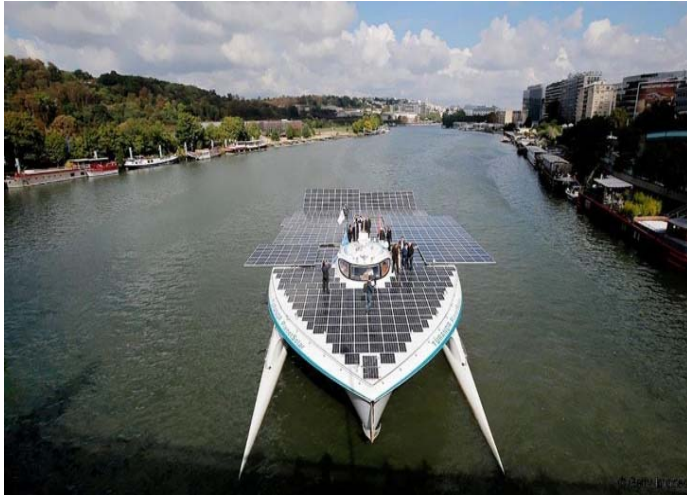
Fig. X, Turanor after achieving its target of circumnavigating the globe powered only by its 512 m 2 solar panels is now operated as a demonstration and scientific platform in the fight against plastic pollution in the oceans. Additionally while in Greece it had another mission as well, an archaeological mission involving the exploration and surveying of a prehistoric settlement in the sea area of Argolid Gulf.
