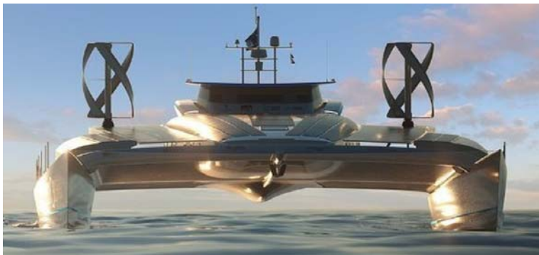
Fig. X, The Energy Observer, a 30m catamaran powered by solar and wind energy will sail around the globe as a floating exhibition and clean energy laboratory. Details about its batteries have not been yet announced.
