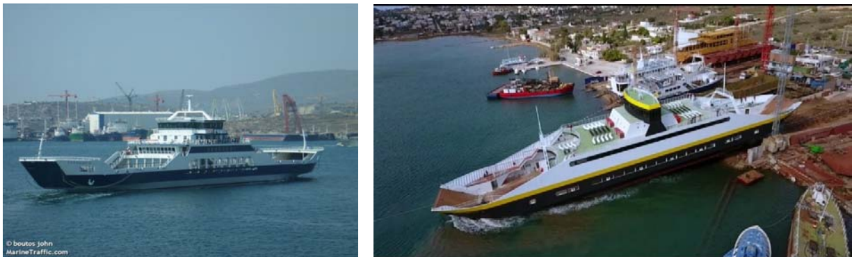
Figure 4-4-1: Photos of typical double-ended Ro/Pax ferry serving Greek waterways
