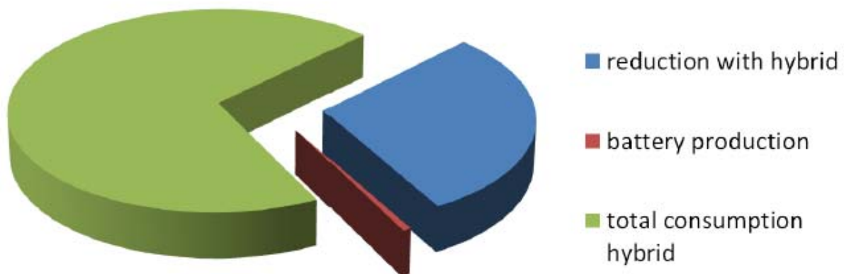
Figure 7-9: Illustration of the distribution of CO 2 emissions for a hybrid ship using 300kWh battery system.
