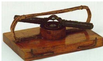
Figure 2-4: Jacobi's first electric motor
