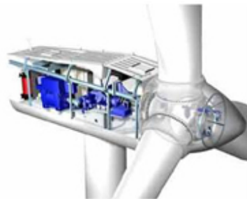
1. Nacelle 2. Heat Exchanger 3. Generator 4. Control Panel 5. Main Frame 6. Impact Noise Insulation 7. Hydraulic Parking Brake 8. Gearbox 9. Impact Noise Insulation 10. Yaw Drive 11. Yaw Drive 12. Rotor Shaft 13. Oil Cooler 14. Pitch Drive 15. Rotor Hub 16. Nose Cone
