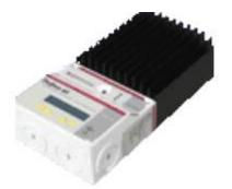
Since the brighter the sunlight, the more voltage the solar cells produce, the excessive voltage could damage the batteries. A charge controller is used to maintain the proper charging voltage on the batteries. As the input voltage from the solar array rises, the charge controller regulates the charge to the batteries preventing any overcharging.
