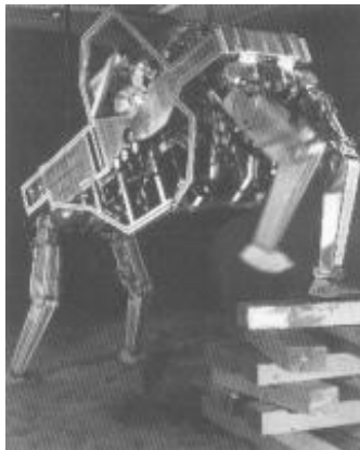
Figure 5-1. General Electric quadruped robot.
