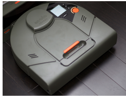
(b) The Neato cleaning robot. Utilizes information from an onboard laser range finder to execute SLAM
