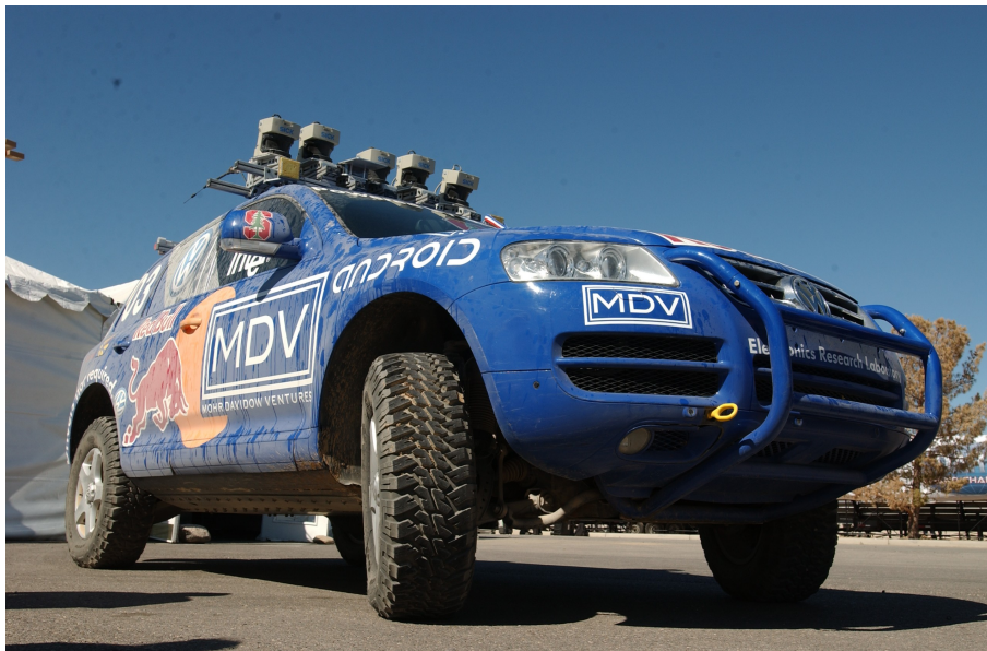
Figure 1.1.2: The STANLEY self-driving car, winner of 2005 DARPA, used SLAM as part of its driving system.
