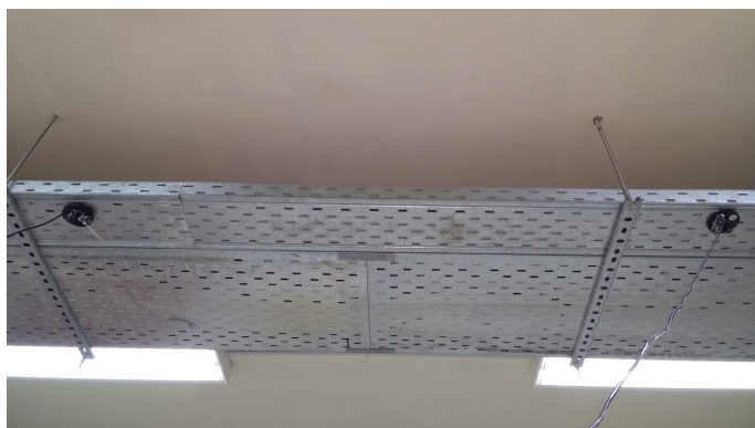
(a) Ceiling cameras used for tracking the Aruco markers. Camera on the left is free to rotate around its axis so a fixed common origin would not be appropriate.
