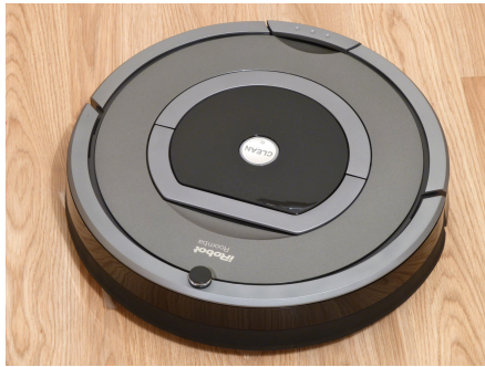
(a) The Roomba cleaning robot. Latest models (most notably the Roomba 900 ) utilize visual SLAM techniques to build a map of their environment.
