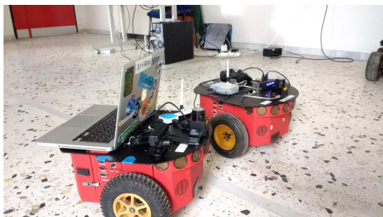
(a) Pioneer 2dx models along with their processing units and data acquisition devices, as used in the multi-robot experiments.
