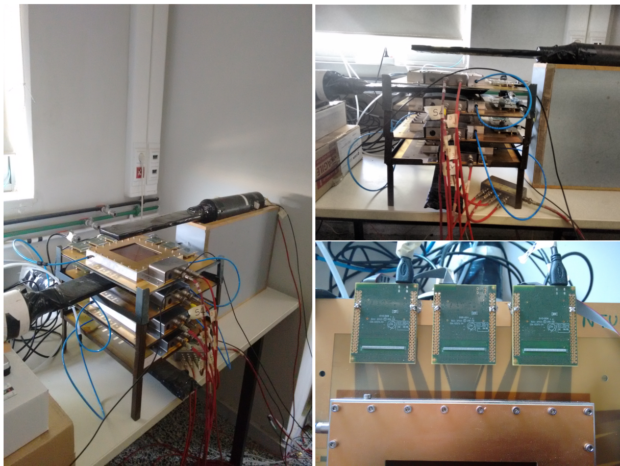
Figure 4.19: Photos of the cosmic muon experimental setup. At the bottom right of the figure, three out of the six APV25 hybrid cards mounted in a Tmm-type MM chamber can be seen.
