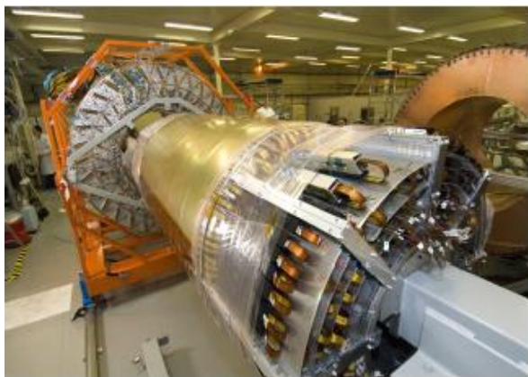
Figure 4.7: Left: The Inner Detector assembly and Right: a representation with the dimensions of the subdetectors. [31]
