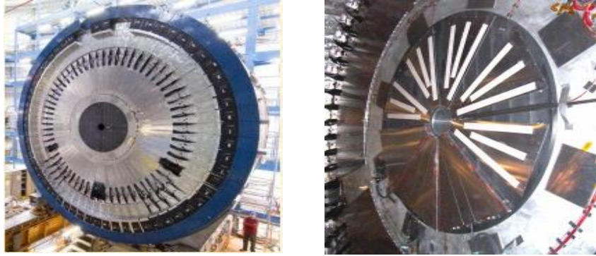
Figure 6.11: Left: The JM after installation on the endcap calorimeter. Right: Installation of scintillators on top of the JM disc. [63]
