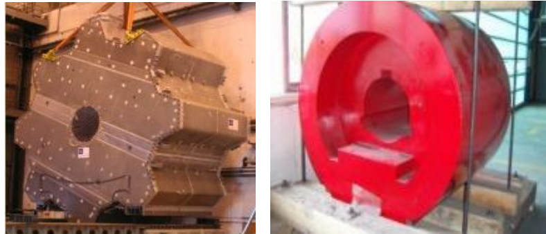
Figure 6.7: The JTT is installed in the hole in the center of the ECT cryostat which is illustrated left. The final JTT ductile iron core pieces are shown at the picture right. [63]
