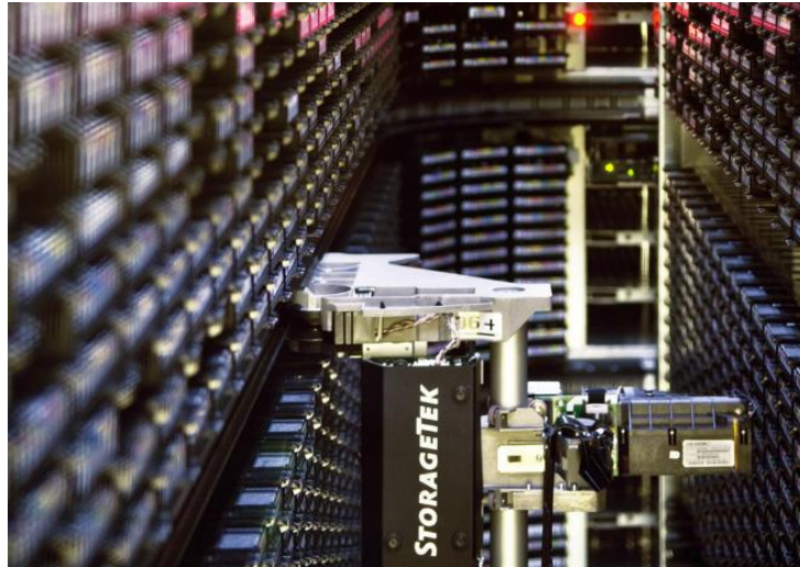
Figure 4.34: A StorageTek machine retrieves server tapes from a stack in the CERN Data Centre. [61]
