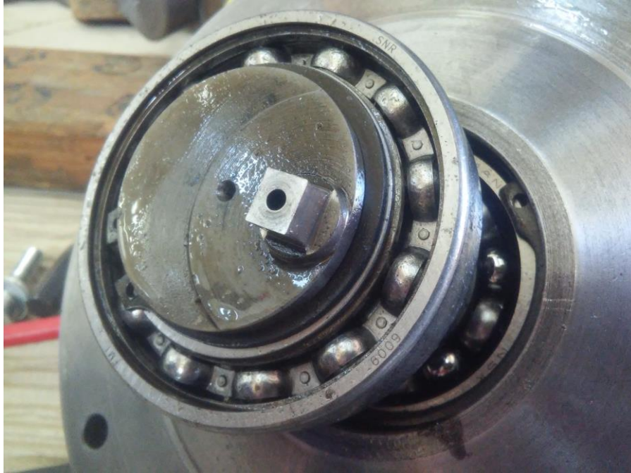
Figure 64 – Damaged “crankshaft” bearing (foreground) and shaft bearing (background).
