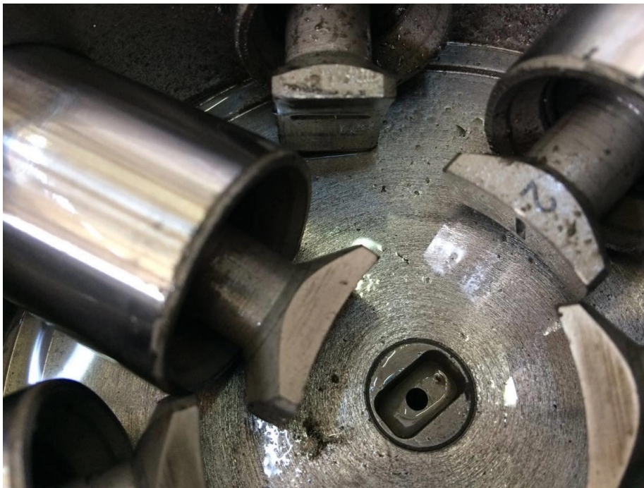
Figure 65 – Iron trims (debris) in the expander interior.
