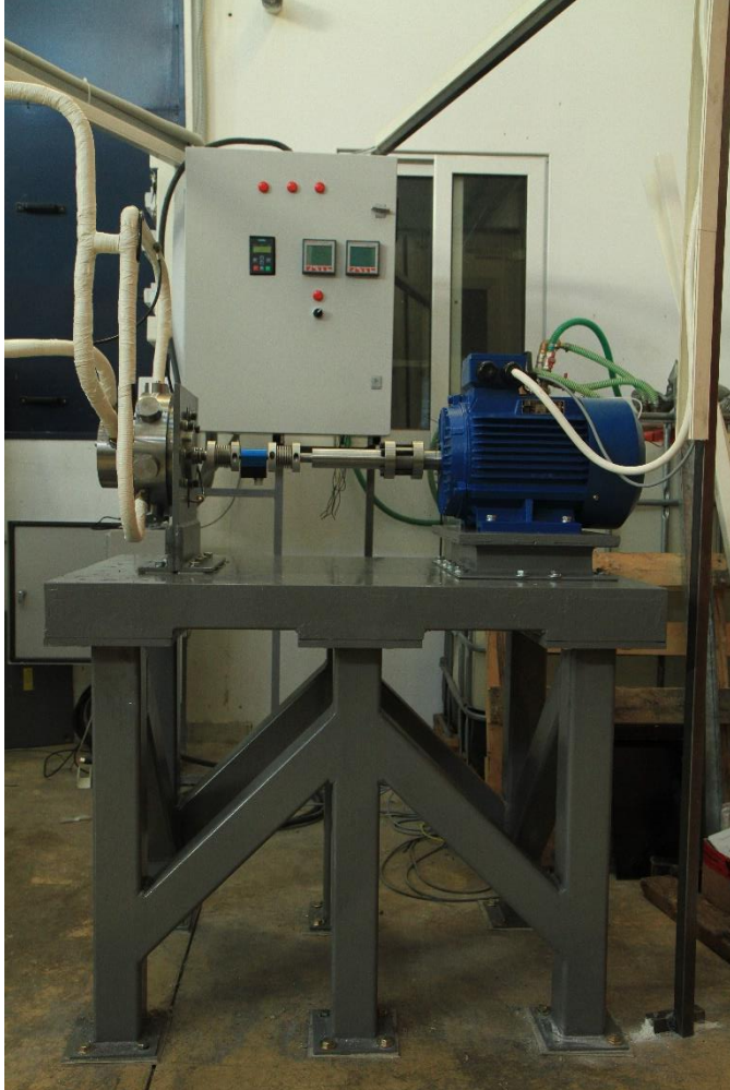
Figure 49 – The dedicated test bench for the mounting of the expander and the generator.
