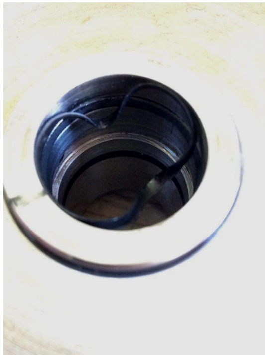
Figure 69 – Deformed shaft O-ring.
