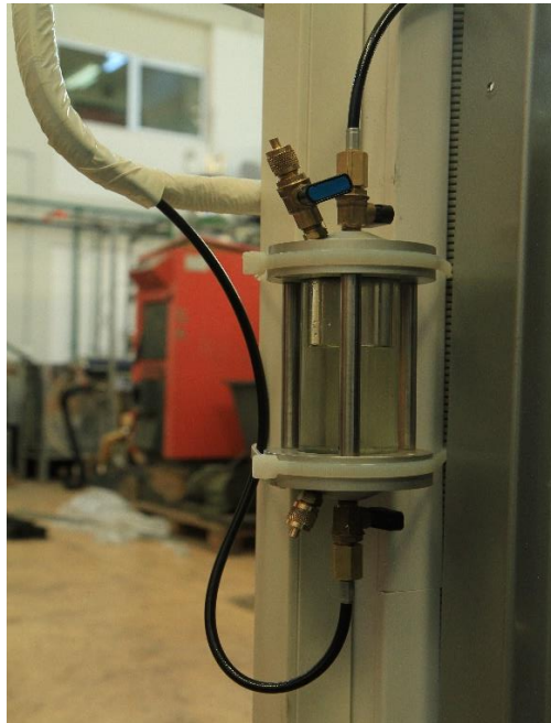
Figure 52 – The heart of expander lubrication system. The depicted oil container is connected with the high pressure circuit of the heat pump at the compressor outlet and this thus pressurized. When its outlet port is open through a dedicated valve the lubricant oil flows into the expander.
