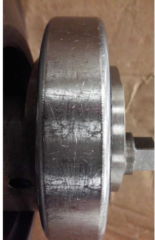
Figure 68 – Scratched surface of crankshaft bearing.
