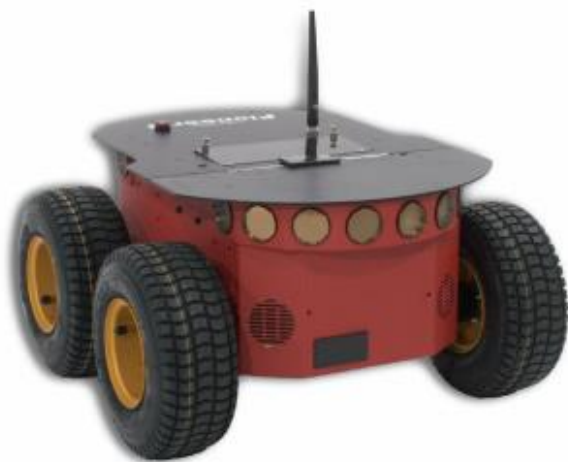
FIGURE 6: PIONEER 2-AT SKID STEERING MOBILE ROBOT. [5]
