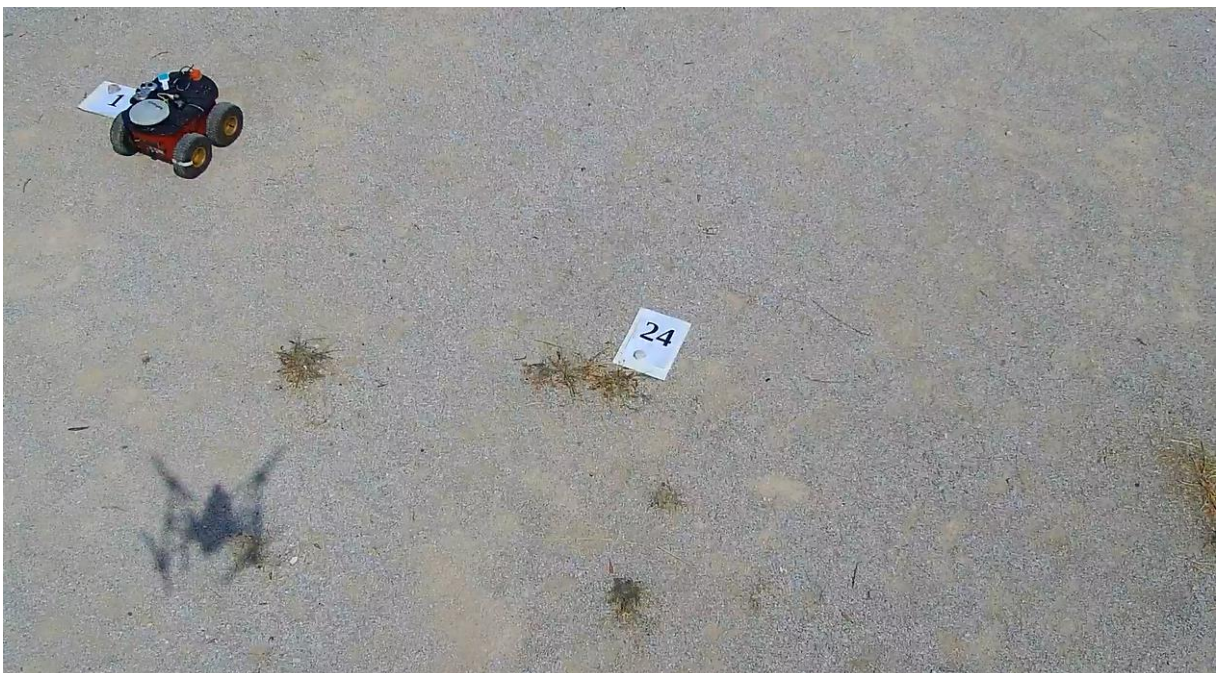
FIGURE 21: SETUP OF EXPERIMENT. THE DRONE RECORDING THE EXPERIMENT CAN BE SEEN AS A SHADOW IN THE PICUTRE. PIONEER 2AT AND TWO CHECKPOINTS CAN ALSO BE SEEN.
