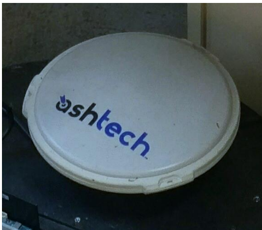
FIGURE 11: GPS ANTENNA PROVIDED FROM THE CSL.
