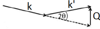
Figure 35: The scattering triangle. \vec{k} and \vec{k}' represent the incident and scattered wavevectors, respectively. The angle between these wavevectors is 2\theta .
