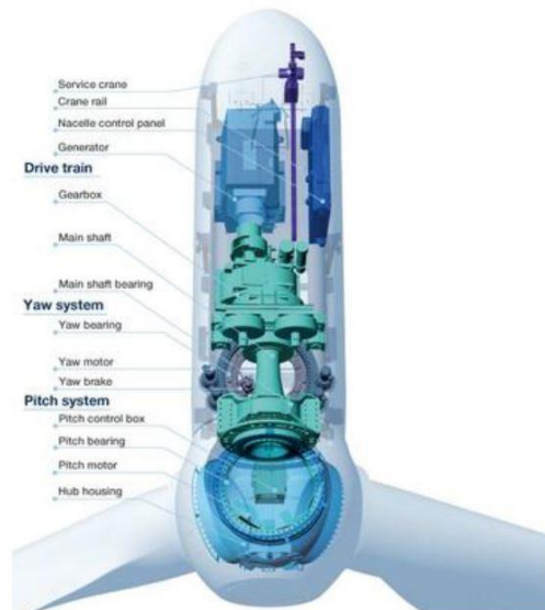
Figure 1.5: Powertrain of a wind turbine. Source: Hitachi
