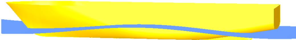
Figure 8.4: RoPax 75 on the wave crest of a wave with  $\lambda=78$  m and  $S_w = 0.0334$
