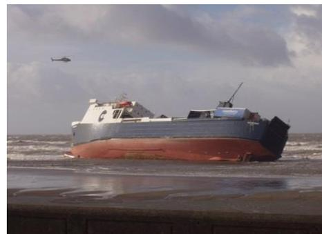
The ship grounded in shore while *passengers and crew members were all rescued*. Accident's investigation [22] showed that pure loss of stability phenomenon was probably liable for vessel's capsized because negative GM was arisen as a wave passed the ship, and the speed of the vessel was slightly slower than waves velocity. It was revealed that master was unaware about IMO Guidance MSC.1/Circ.1228
