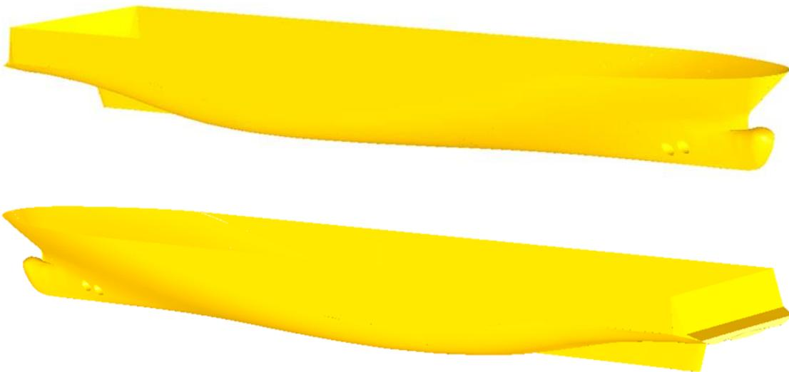
Figure 6.1: Render views of the hull-form of RoPax 160
