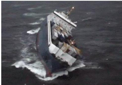
Sea on 1 November 2006 during a trip from Helsinki (Finland) to Aarhus (Denmark). In her last voyage Finnbirch was loaded with semi-trailers and a consignment of block stowed paper reels. The weather was hard with winds at 20 m/s and gusts up to 26-29 m/s. Significant wave height was approximately 4 m with a dominant period of 6.7 sec. Individual waves can therefore had reached a height of approximately 7-8 m. The ship was sailing at a speed of 17.5-18.5 kn in
