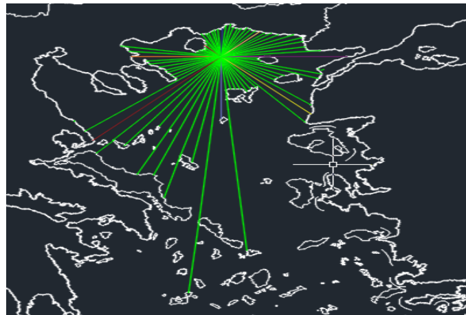
Figure 3.2 Fetch lengths around the study point
