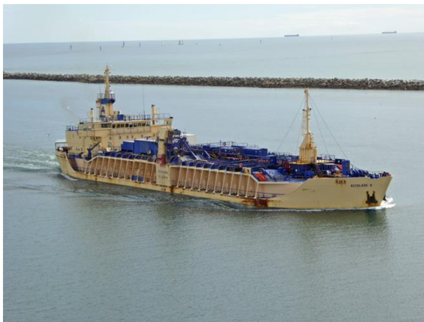
Figure 1-4 The 8140DWT limestone carrier "Accolade II" (L=108m, B=23m, T=6.1m) (ShipSpotting.com, 2015a)
