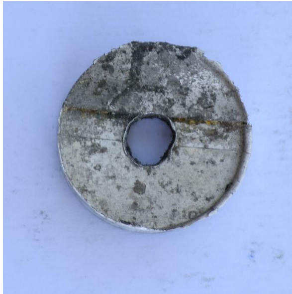
Figure 3-18 The internal surface of the specimen cut from the aluminium liner at the dome-cylinder joint. The line in the middle is where the joint is. The dark surface is at the dome region and the lighter surface at the cylindrical portion.
