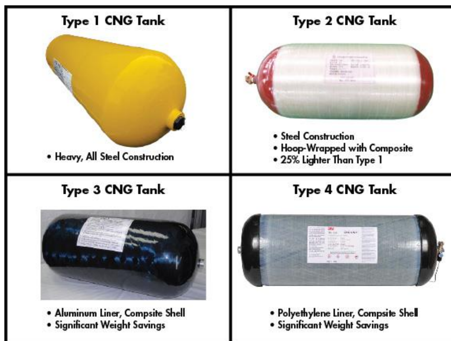
Figure 2-2 Schematic representation of the four types of pressure vessels and their main characteristics (Dillard, 2015)
