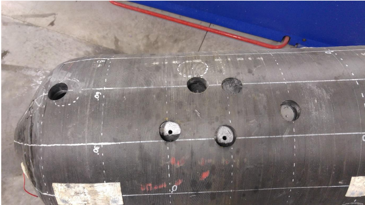
Figure 3-15 Various holes made with a hole saw in order to measure the thickness of CFRP at the cylindrical portion of the pressure vessel. At the left of the picture, the hole, where the starting point of the dome was verified, can be distinguished. The white lines shown divide the pressure vessel in different location areas.
