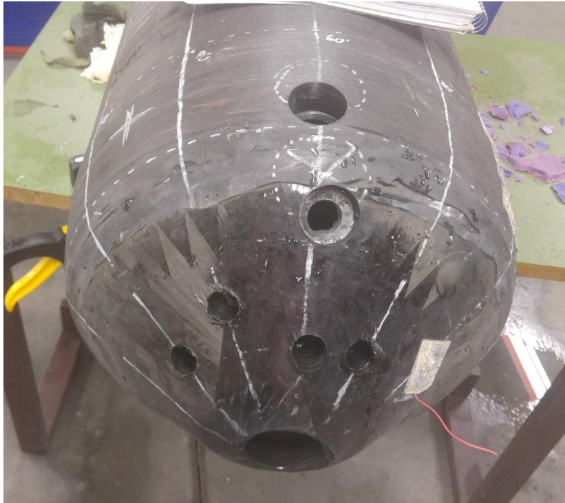
Figure 3-19 The five holes, which were made at the dome region. The first was made with a hole saw, whereas the rest of them with a drill.
