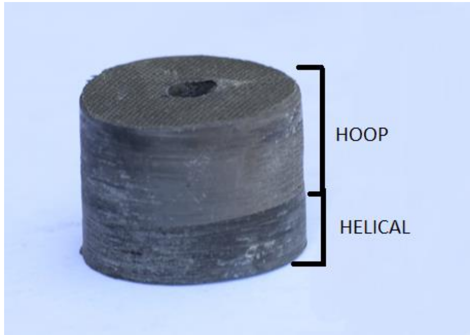
Figure 3-16 Photo of a specimen of CFRP from the cylindrical portion of the pressure vessel
