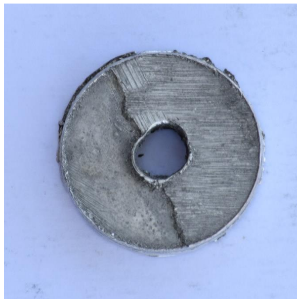
Figure 3-17 The external surface of the specimen cut from the aluminium liner at the dome-cylinder joint. The line in the middle is where the joint is. The surface at the right (roughened surface) is at the dome region, whereas the left surface (polished) is at the cylindrical portion
