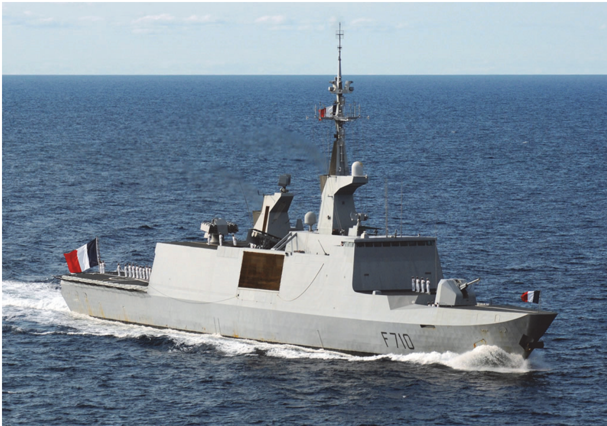
Fig. 1.5. La Fayette class frigate of the French Navy. Among the first large warships fitted with a composite superstructure. In particular, the aft section of the superstructure, including the helicopter hanger, is made of GRP-sandwich composite panels.
