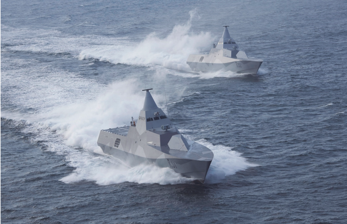
Fig. 1.3. Two Visby-class corvettes of the Swedish Navy built from sandwich composite panels having face skins of hybrid carbon- and glass fiber polymer laminate covering a PVC foam core.
