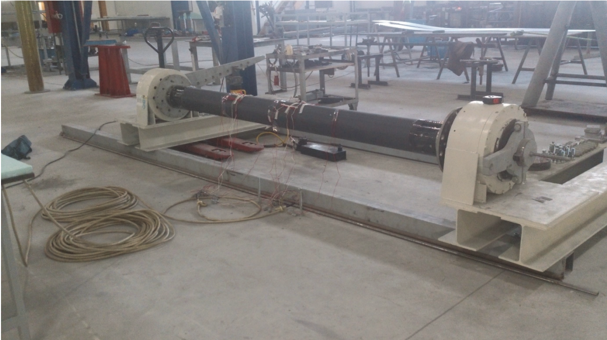
Fig. 3.3. The CFRP shaft fitted to the torsion fixture
