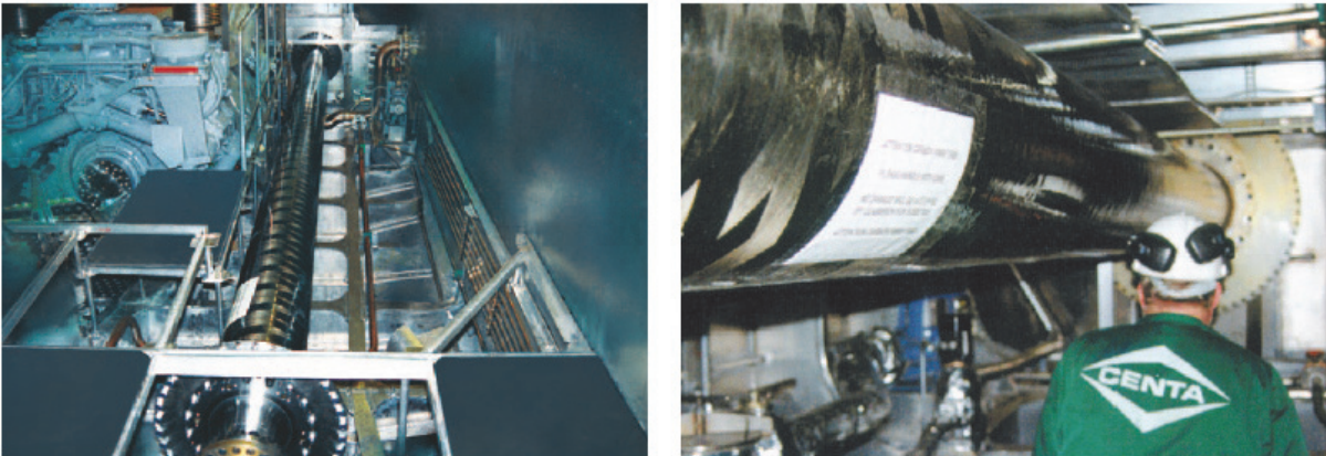
Fig. 1.10. CENTA carbon fiber shafts in “Flying Cat” (left) and “Jumbo Cat”(right) catamarans
