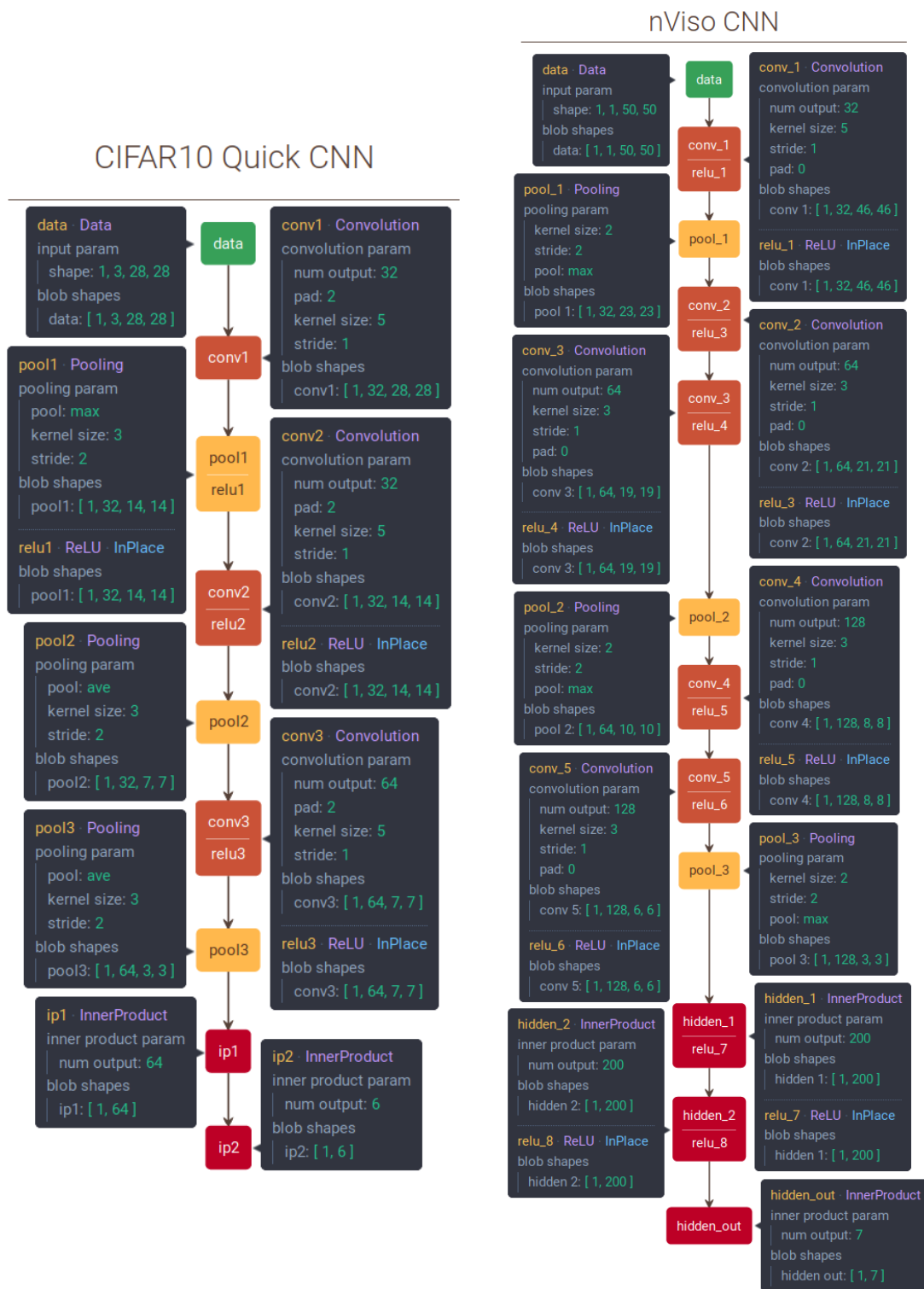
Figure 6.1: Left: CIFAR10 Quick CNN for terrain classification. Right: nViso CNN for emotion classification from facial expressions.
