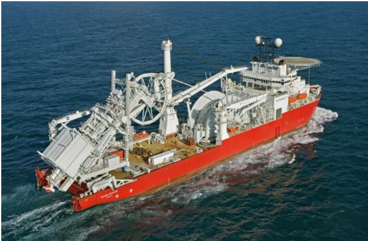
Figure 2.7 400 mt Reel-Lay System Seven Ocean, Subsea 7 [Jensen, 2010]
