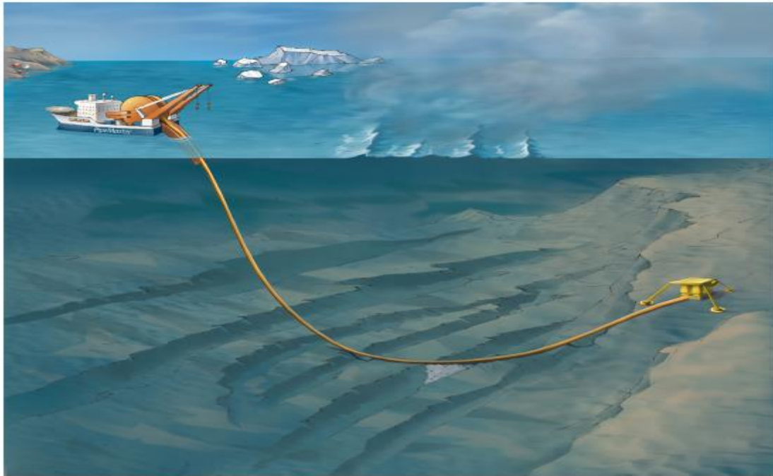
Figure 2.4 Offshore pipe laying operation [Stenberg, 2009]
