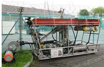
Figure 4 A Royal Navy ROV ( Cutlet ) first used in the 1950s to retrieve practice torpedoes and mines
