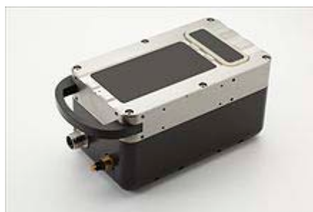
Figure 1 A multibeam echosounder showing the transmit array (larger black rectangle) and receive array (narrower rectangle) - Odom MB1
