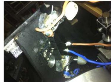
**Figure 2.3.1.8.1** Successive holder improvements, using sharper probes and double-side access. The probes are positioned on the front side, while the light beam is focused at the back side through a hole drilled in the holder base.
