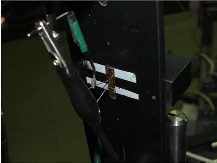
**Figure 2.3.1.2.8** Final setup close view of the contacted diode exhibiting EL, also in the visible spectral range.
