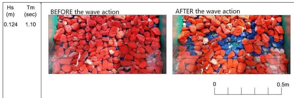
Figure 8: Eroded area after regular wave attack ( H_s=0.124\text{m} , T_m=1.10\text{sec} ) with duration t=10\text{min}
