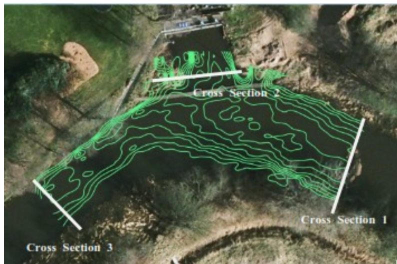
Figure 4.3-2: Contour lines of depth average velocities in the area of Jedsted Mill Fish Farm. Cross sections at the inflow and outflow location are shown with white straight lines [Source: (Jon C. Svendsen, after personal communication)]
