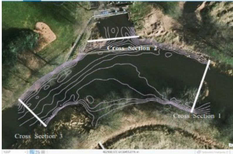
Figure 4.3-1: Contour lines of water depth in the area of Jedsted Mill Fish Farm. Cross sections at the inflow and outflow location are shown with white straight lines [Source: (Jon C. Svendsen, after personal communication)]
