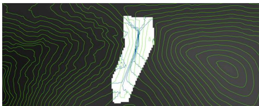
Figure 5 Influence of the terrain to the given output of focal statistics geoprocessing for gappfilling. Blue contours show the output generated from a rectangular neighbor, while green contours show the one generated from an elongated neighbor feature.
