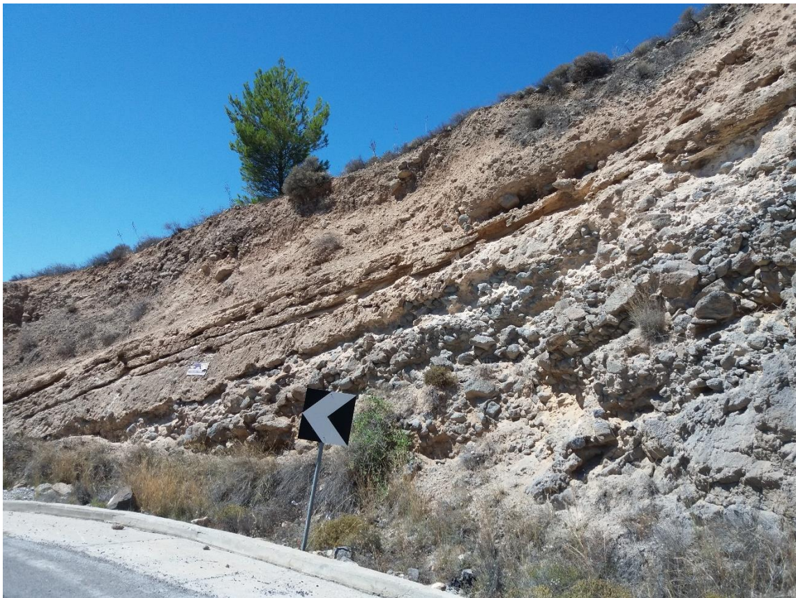
Figure 3.6: Sedimentary rock horizontally jointed with horizontal continuity and vertical heterogeneity (Aegina, Greece)
