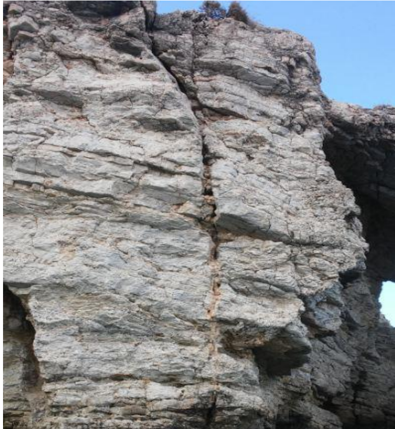
Figure 3.8: Slope in rock mass crossed by vertical joint normal the slope face, which do not affect the slope stability (Kythera, Greece)
