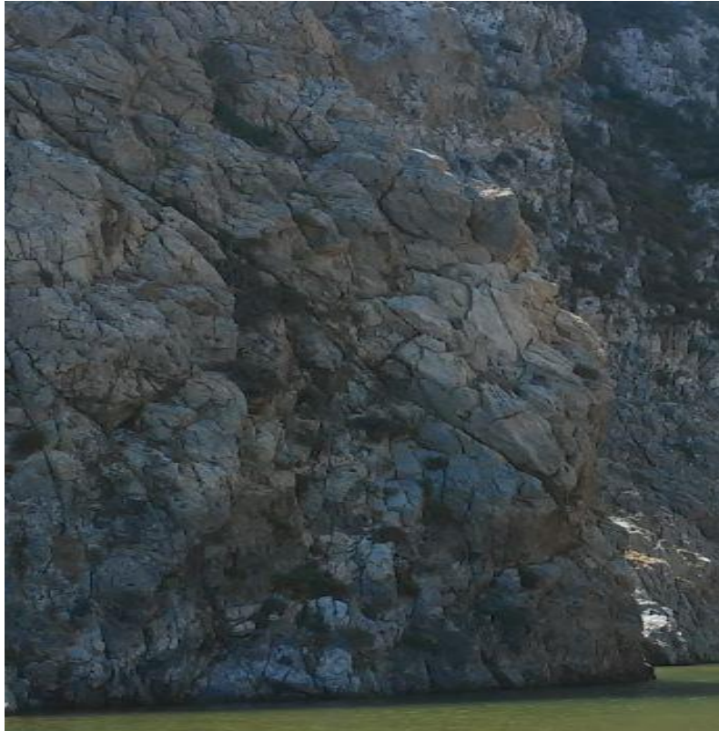
Figure 3.9: Slope in rock mass crossed by an oblique joint, which can affect the slope stability (Kythera, Greece)
