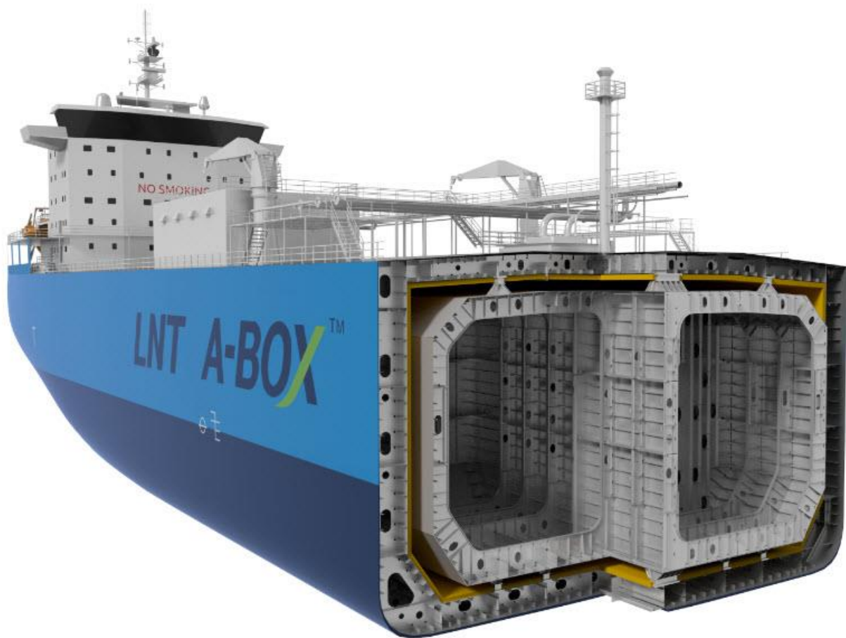
Picture 3-7 Section view of and LNG showing the internal space of the specially-built tank (“Xiamen Bags First LNG Carrier Order | World Maritime News,” 2015)
