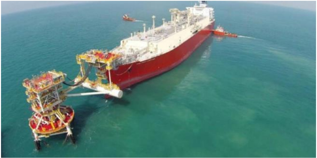
Picture 4-10 Yoke system mooring (Manos Migadis, 2017)
