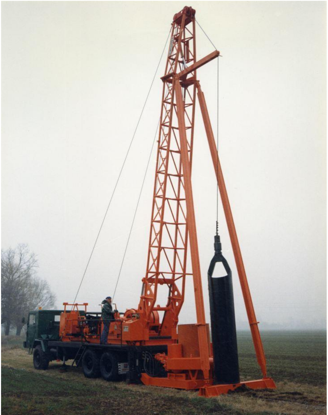
Picture 3-3 A Modern, Mobile Cable Tool Drilling Rig (“What is percussion well drilling method - Massenza Drilling Rigs,” 2017)
