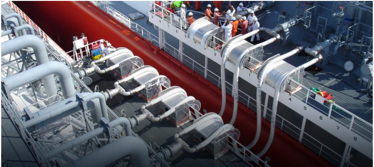
Picture 4-5 STS flexible hoses (“Excelerate Energy – STS LNG Transfer,” 2017)
