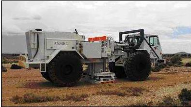
Picture 3-1 ANSIR vibrator seismic energy source "Brolga", 60,000 pounds pressure ("Deep seismic profiling of the earth's crust in Australia: startup, 1950s and 1960s - Historical Data - IGCP Project 599, Crustal Architecture and Images," 2016)
