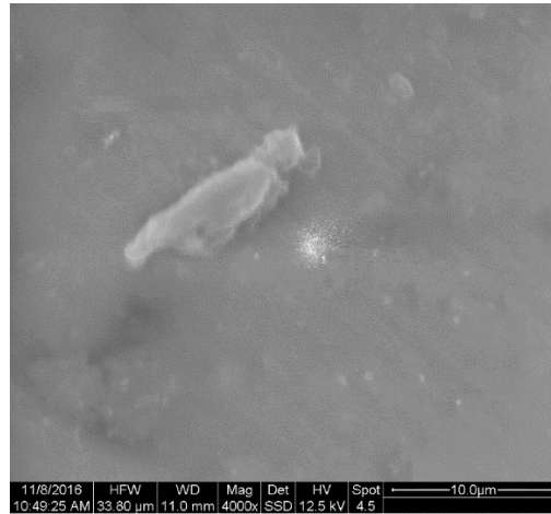
Figure 1.2. Graphene nanoplatelet (GNP) in the epoxy matrix (Seretis et al. 2017a).
