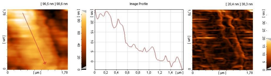
Figure 5.7. AFM micrographs showing the linear height profile of a GNP after sonication time 20 min as well as the GNP boundaries using an edge detection filter (Seretis et al. 2018).
