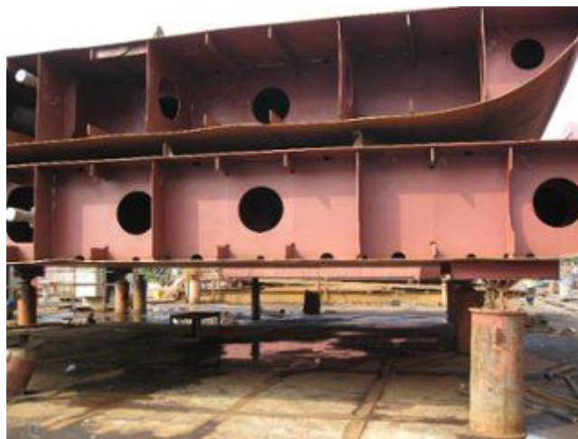
FIGURE 2.1: Double bottom of a vessel.
