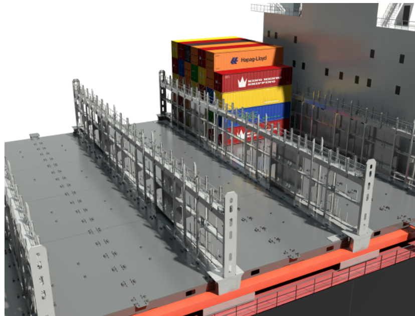
FIGURE 2.3: A view of the upper cargo area of a container vessel; cell guides, hatch coamings and hatch covers.
