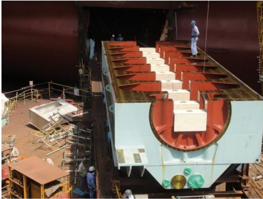
FIGURE 2.5: Engine bedplate of a marine diesel engine.
