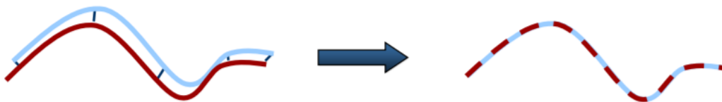
Figure 5-3: ICP converges when the starting positions are “close enough”
