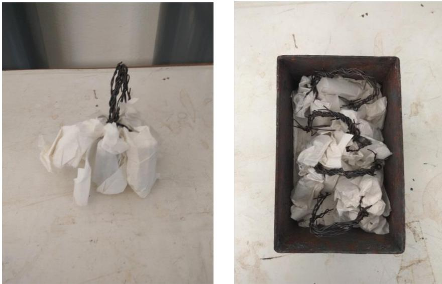
**Fig.38** The specimen are wrapped in filter paper inside the box
