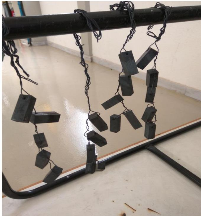
**Fig. 36** Grouped specimens before inserting in furnace
