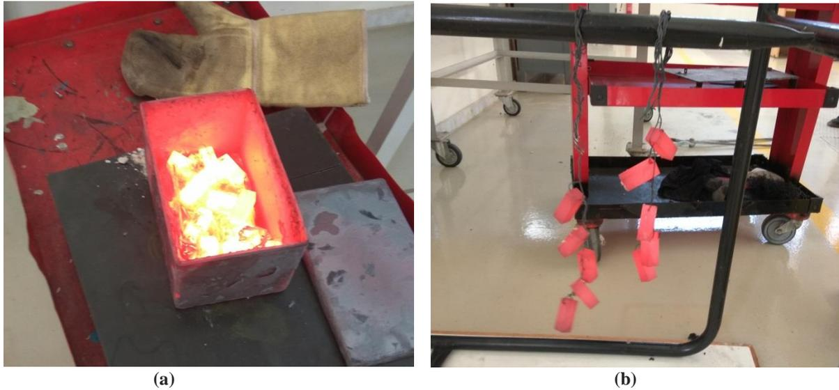
**Fig 40.** (a) The box of specimens out of the furnace, (b) The specimens ready for quenching
