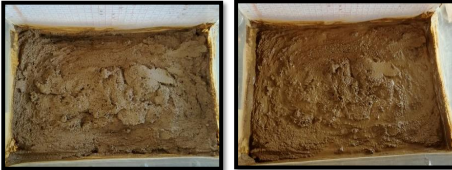
Figure 55 a, b The sample with 27.9% moisture content before and after the sway experiments. The movement of the whole sample was now a lot more intense.
