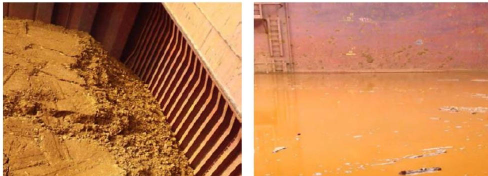
Figure 9 Photos of dry and liquefied ore inside the cargo holds (Roxburgh Environmental Ltd)
