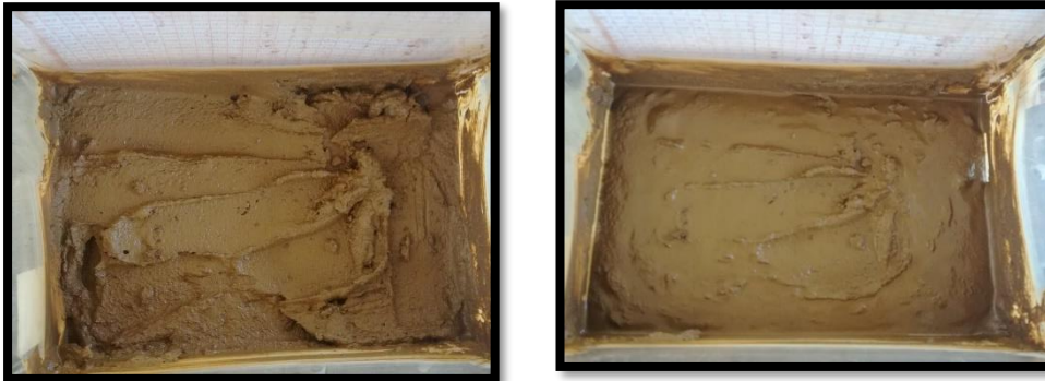
Figure 59 a, b The sample with 33.3 % moisture content before and after the sway experiments.
