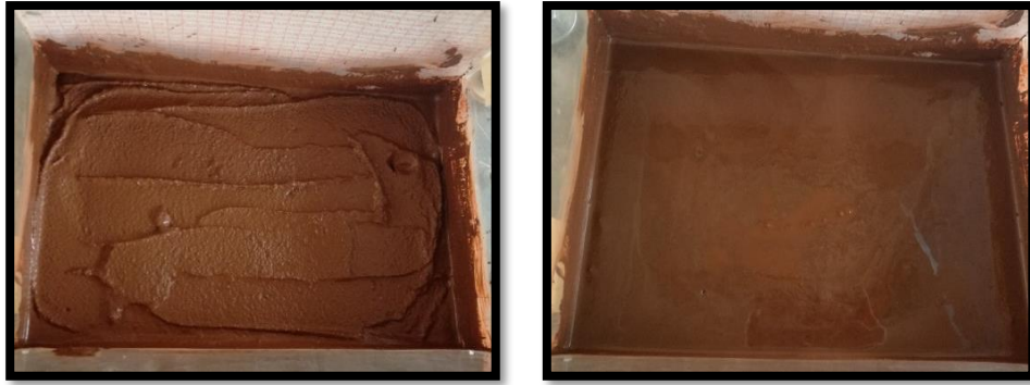
Figure 39 Sample with 22.5% moisture content before and after the roll experiments
