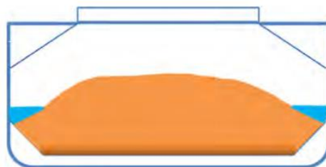
Figure 23 Initial stage of cargo instability due to dynamic separation (Global Bauxite Working Group, 2017, p. 83)
