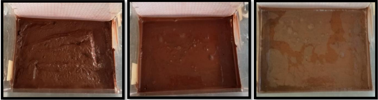
Figure 37 a,b,c Sample with 20.3% of moisture content before and after the experiments of roll movement turning into a muddy material. Also in the last photo can be observed the sample the next morning in which the water seems to have been raised in the surface.
