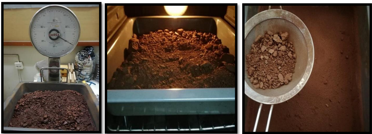
Figure 33 a, b, c Weighing, drying and shifting the sample of Nickel Ore
