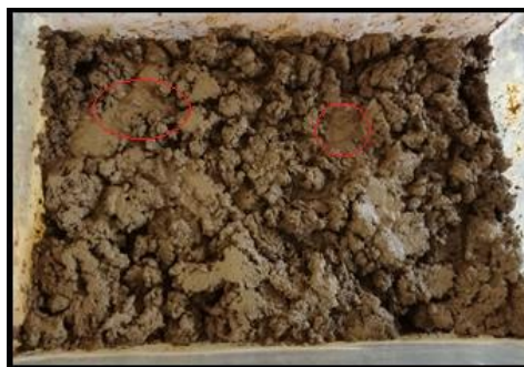
Figure 49 After one hour of sway motion at 1Hz some unimportant spots of water can be observed.
