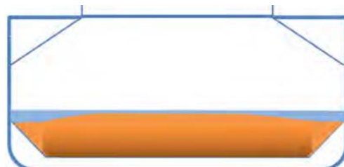
Figure 24 Final stage of cargo instability due to dynamic separation (Global Bauxite Working Group, 2017, p. 83)
