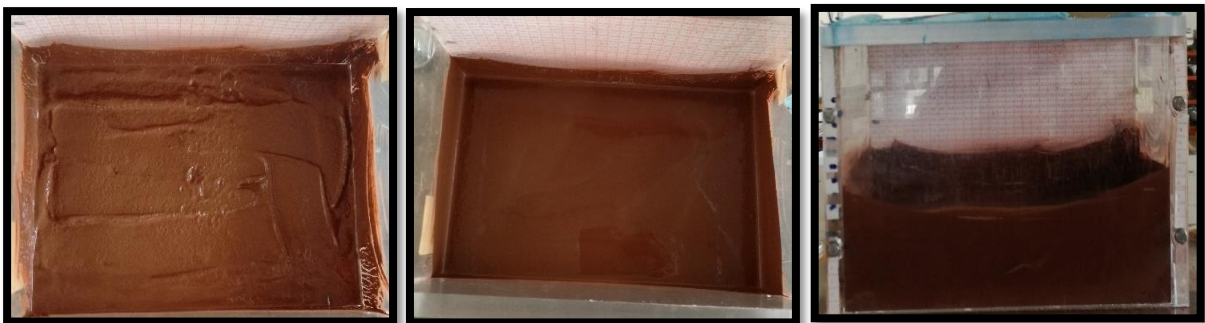
Figure 40 a, b, c Sample with moisture content 25.35% before , during and after the sway experiments. It can be seen that inside the tank during the experiments the sample is shifting from the one side to the other.
