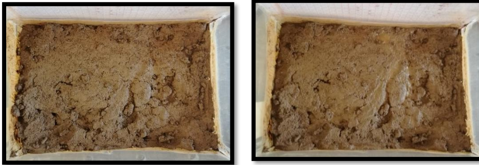
Figure 53 a, b Sample with 23.42% moisture content before and after the sway experiments.
