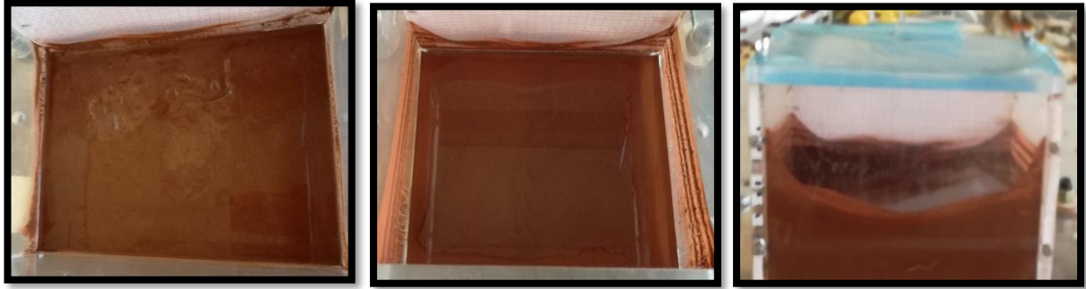
Figure 47 a, b, c Sample with 31,7% moisture content before, during and after the sway experiments. The sample even before the experiments looked watery and it behaved like that during the experiments.
