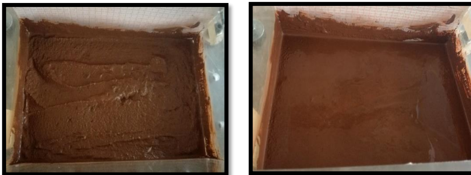
Figure 38 a, b Sample with 22.5% moisture content before and after the sway experiments
