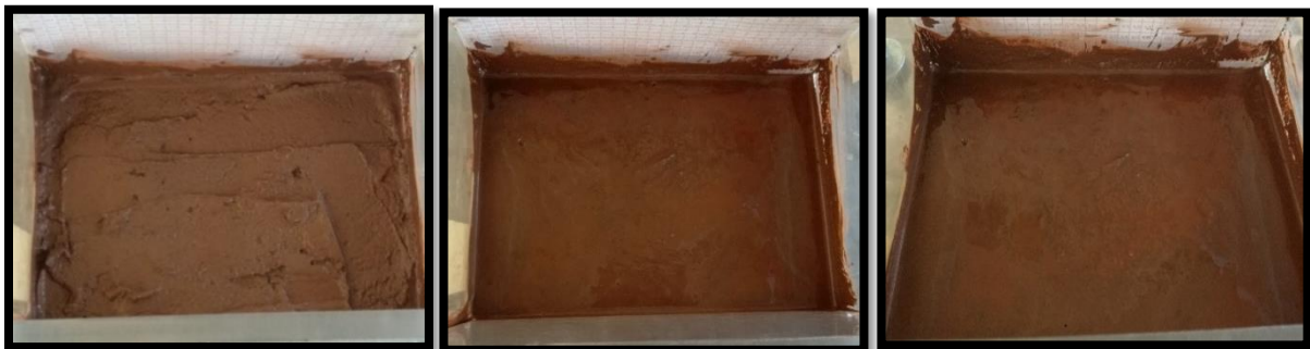
Figure 36a, b, c Sample with 18.3% of moisture content before and after the heave experiments turning into a muddy material.
