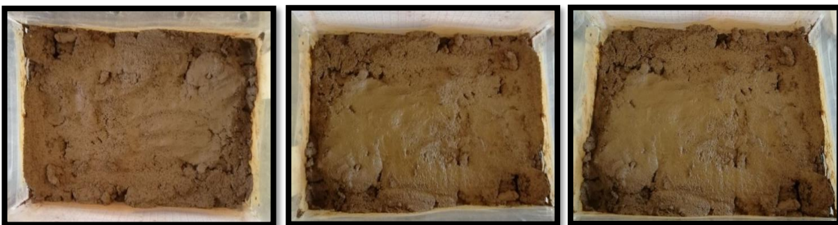
Figure 52 The sample with 21.6% of moisture content before and after the sway experiment at 1.2Hz. No difference could be observed in the sample.
