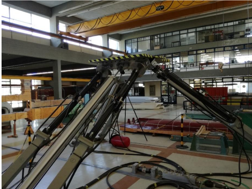
Figure 31 The shaking table in the School of Naval Architecture and Marine Engineering.
