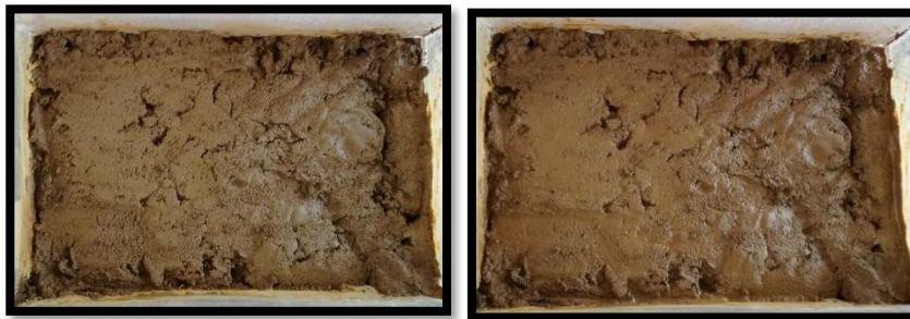
Figure 51 The sample with 21.6% of moisture content before and after the sway experiment at 0,8Hz. No difference could be observed in the sample.
