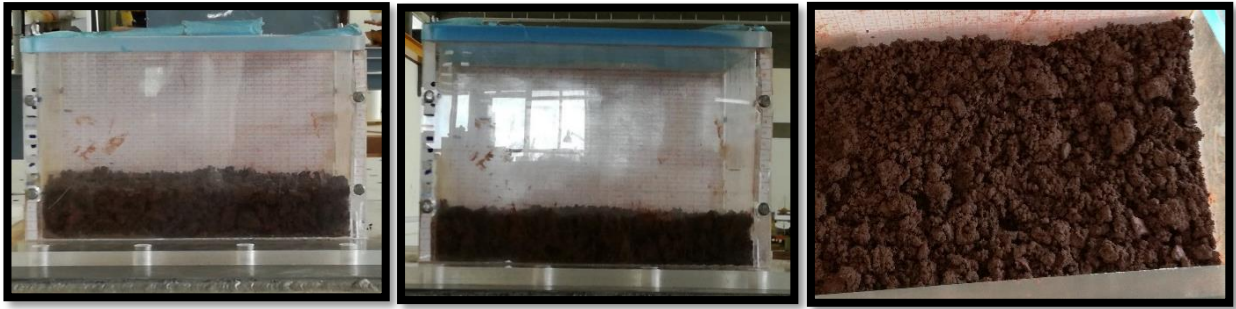
Figure 35 a, b, c The wet sample of Nickel Ore before and after the compaction.
