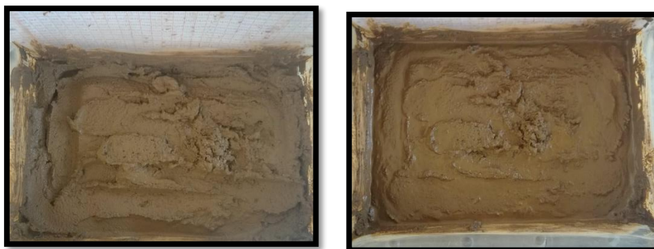
Figure 57 a, b The sample with 29.7% moisture content before and after 1 hour of sway experiments.
