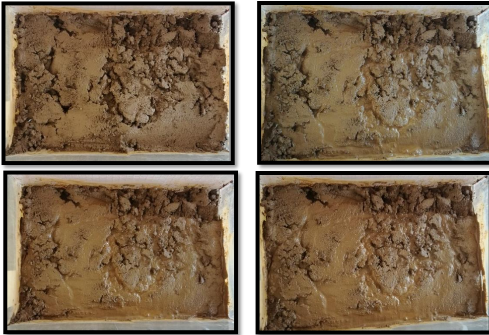
Figure 50 a, b, c, d The sample with 21.6% moisture content at the beginning of the sway experiment at 1Hz, after 20 minutes, after 40 minutes and after 1 hour.
