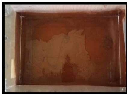
Figure 42 The sample after hours of being stored in the tank. The water that was inside the sample created a lake on the top of the drier sample.
