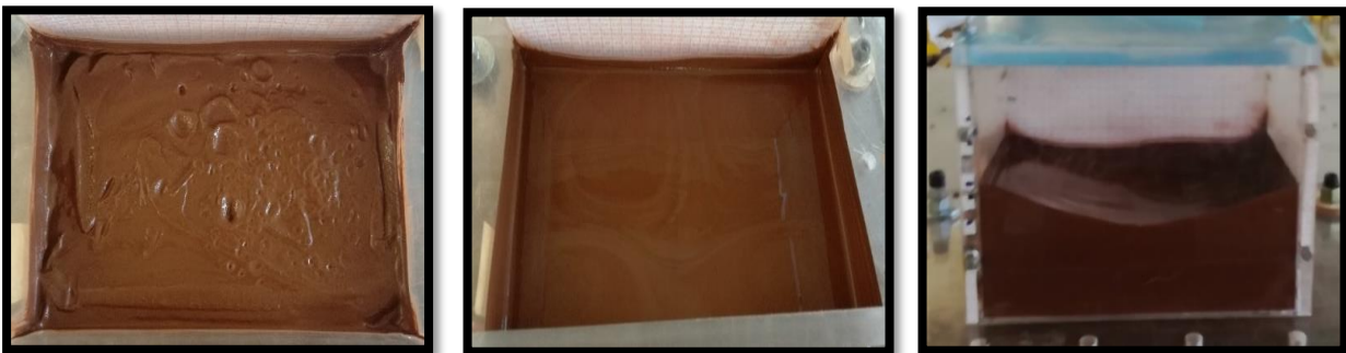
Figure 44 a, b, c The sample with 28.17% moisture content before and after the roll experiments
