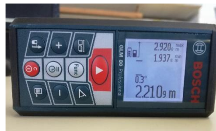
Figure 32 Photo of the laser that was used for the calibration process
