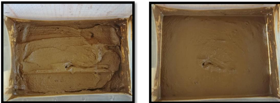
Figure 60 a, b The sample with 36% moisture content before and after the sway experiments. The whole sample behaved like a muddy thick liquid.
