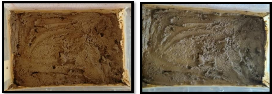
Figure 54 Sample with 26% moisture content before and after the sway experiments.
