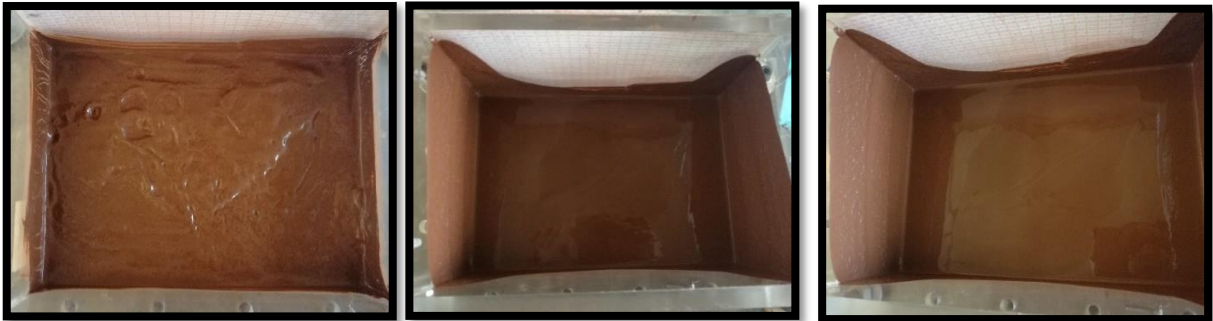
Figure 43 a, b, c The sample with 28.17% moisture content before and after the sway experiments. As it can be seen in the last photo the sample was shifting in the whole height on the sides of the tank.
