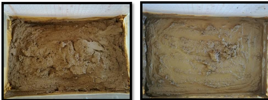
Figure 56 a, b The sample with 27.9% moisture content before and after the roll experiments. The amount of water that could be observed in the surface was more than after the sway experiments.
