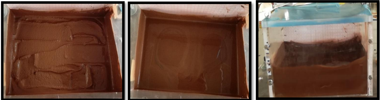
Figure 41 a, b, c Sample with moisture content 25.35% before , during and after the roll experiments. Sample was behaving like a liquid.
