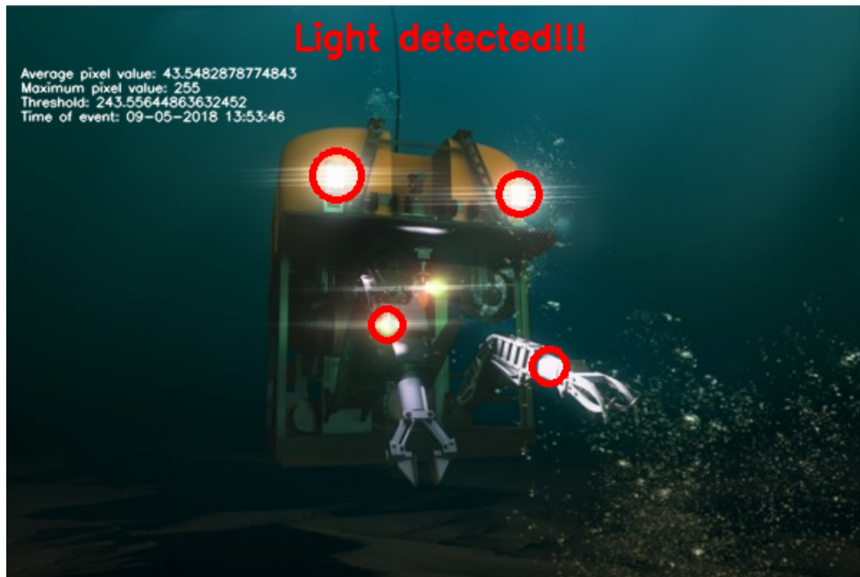
Figure 5.3: Light detection in Image with ROV
