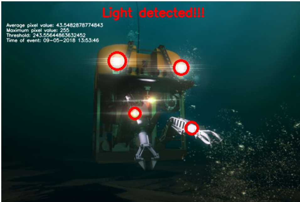
Figure 4.4: Light detection in Image with ROV
