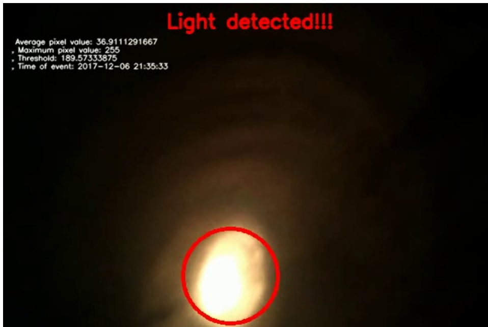
Figure 5.5: Light detection in very dark environment
