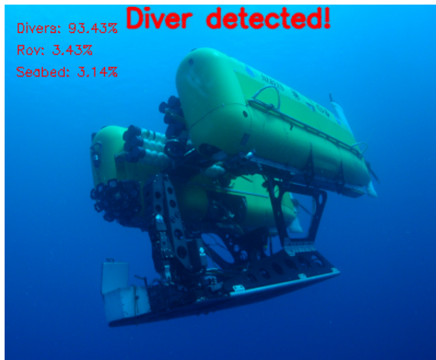
Figure 5.17: False classification of a ROV
