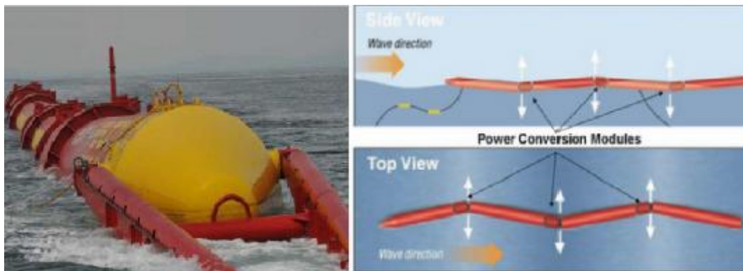
Figure 1.6: Attenuator-the Pelamis (Sinha 2015).
