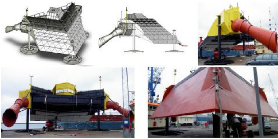
Figure 1.8: Overtopping: the wave plane (WavePlane 2010).
