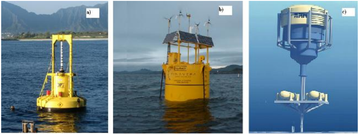
Figure 1.9 Point absorbers: (a) the Powerbuoy, (b) the Aquabuoy and (c) the AWS. (Sinha 2015).
