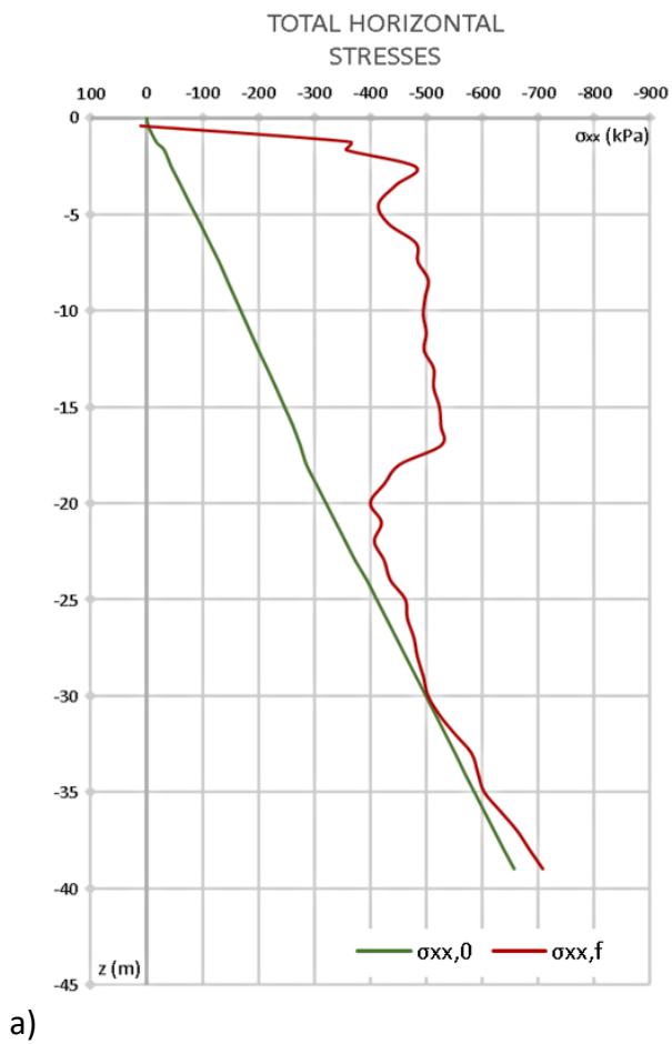
Figure 3.24 Distribution of a) total horizontal stresses and b) additional horizontal stresses with depth for 95%G, 90% S_u
