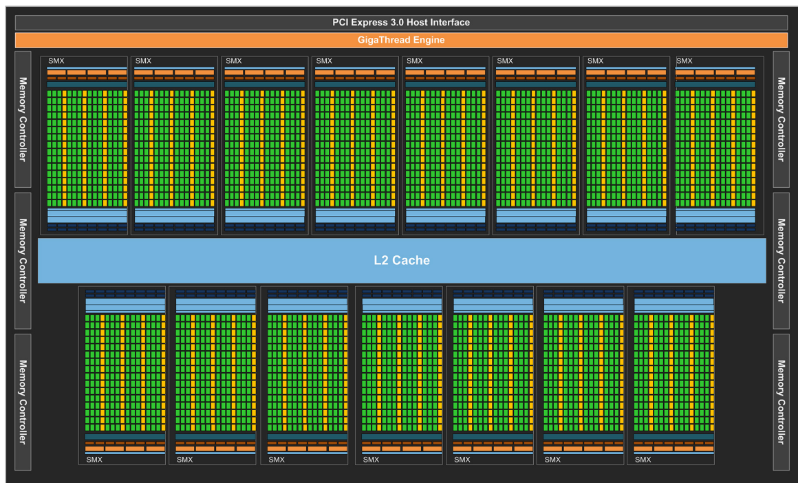
Figure 1.3: The Kepler architecture. source: Nvidia CUDA programming guide
