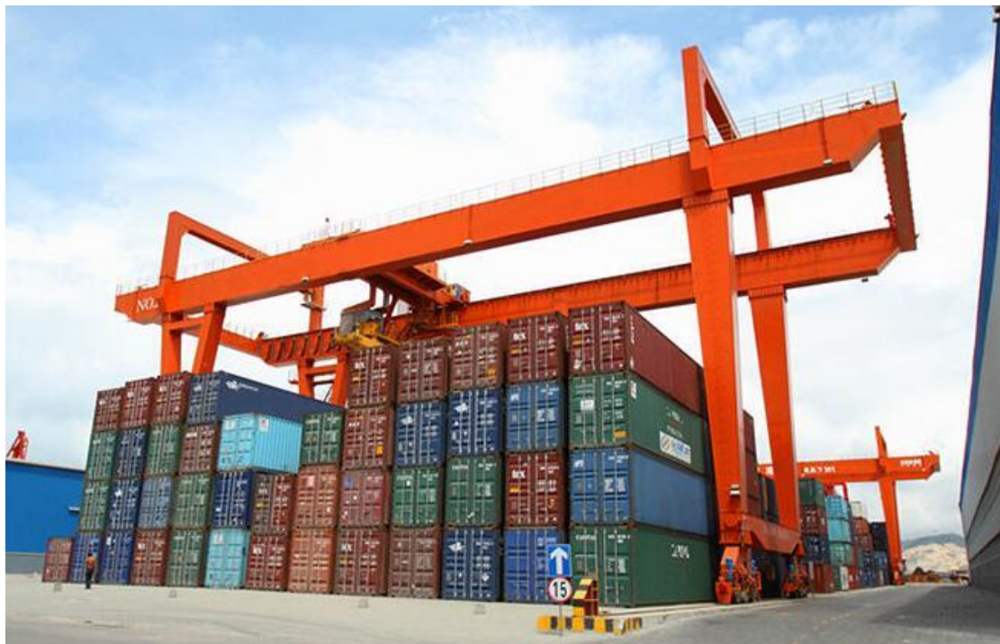
Figure 8. Railed Mounted Gantry Cranes (Lincolnmcs)
