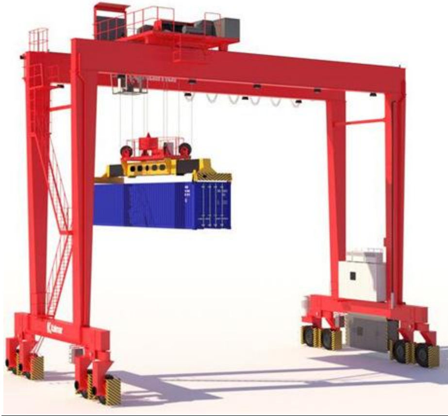
Figure 9. Rubber Tired Gantry Crane (Apdisplay)
