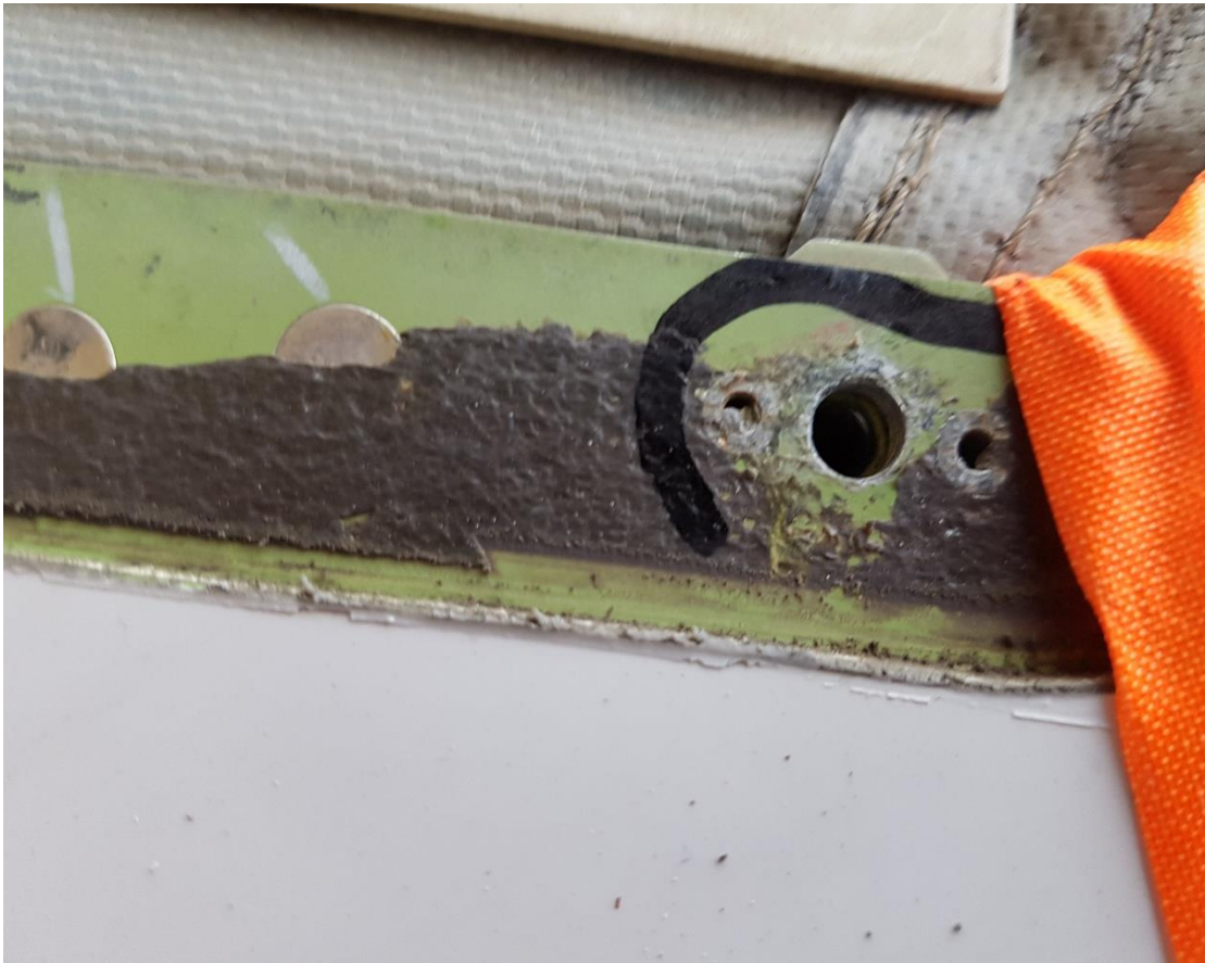
Photo 5.2f: Corrosion horizontal stabilizer
