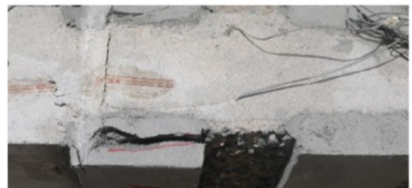
(b) P-F-F (FRCM composite removed)
