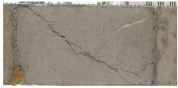
(b) P-F-F (FRCM composite removed)
