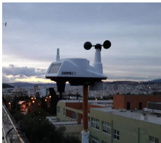
Figure 3.5 The Davis Vantage Vue weather station sighted on the rooftop of the SRSE.
