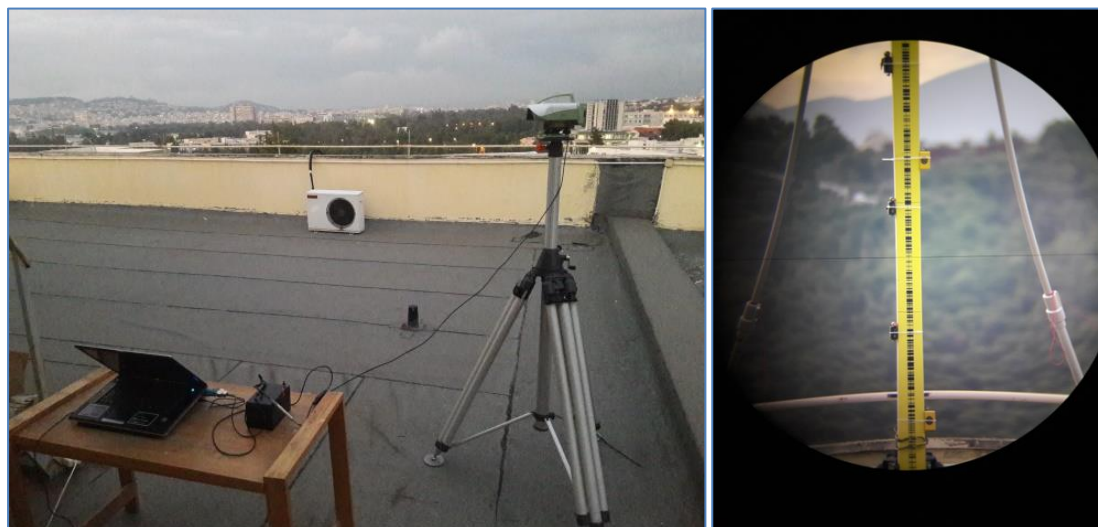
Figure 4.17 The instrumentation set up of the outdoor experimental tests at 40m, the automatic online command of the digital level (left) and the level's focusing on the bar coded staff (right).
