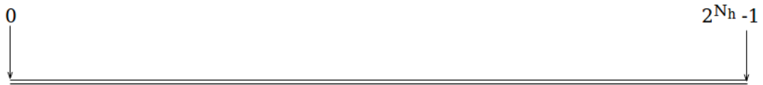
Figure 3.7: An axis on which all possible outputs of the N_h -bit hash function can be conceptually “placed”, thus representing the whole keyspace.
