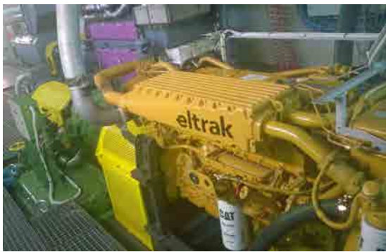
Fig. 10. Hybrid integrated propulsion powertrain on which all the measurements and experiments presented in the paper are performed. Caterpillar 3176B (dark yellow), water-brake (dark green) and the induction motor (gray) are shown. The cardan shafts connecting the powertrain are covered with the yellow colored casings.
