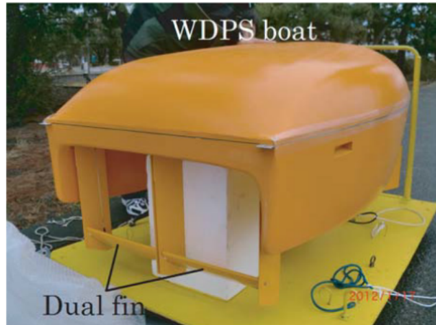
Figure 1.6: Terao and Sakagami (2013) equipped an small autonomous boat, for ocean measurements, with a wave devouring propulsion system (WDPS).
