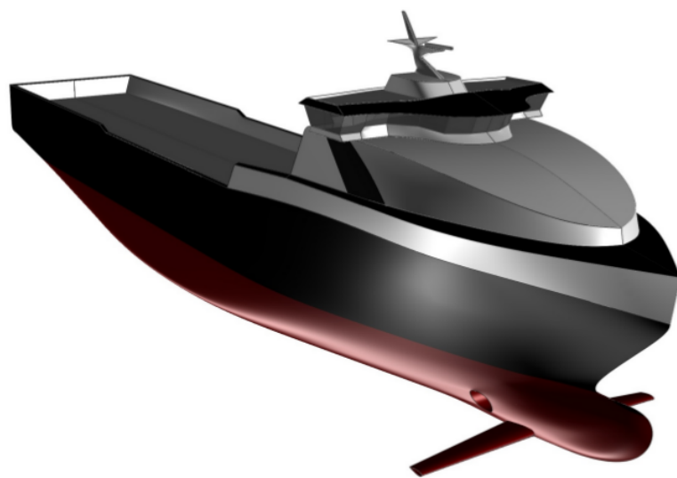
Figure 1.9: The case vessel with wavefoils deployed from work Bøckmann et al. (2018) were fuel savings from the wave-foils were estimated.
