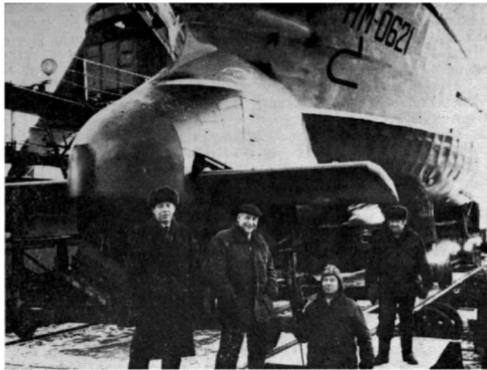
Figure 1.4: Russian research fishing vessel equipped with flapping foil (Nikolaev et al. 1995).
