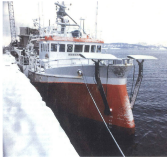
Figure 1.2: Jakobsen equipped fishing research vessel Kystfangst, owned by the Institute of Fishery Technology Research, with a bulbous bow and two foils on each side of the bow.
