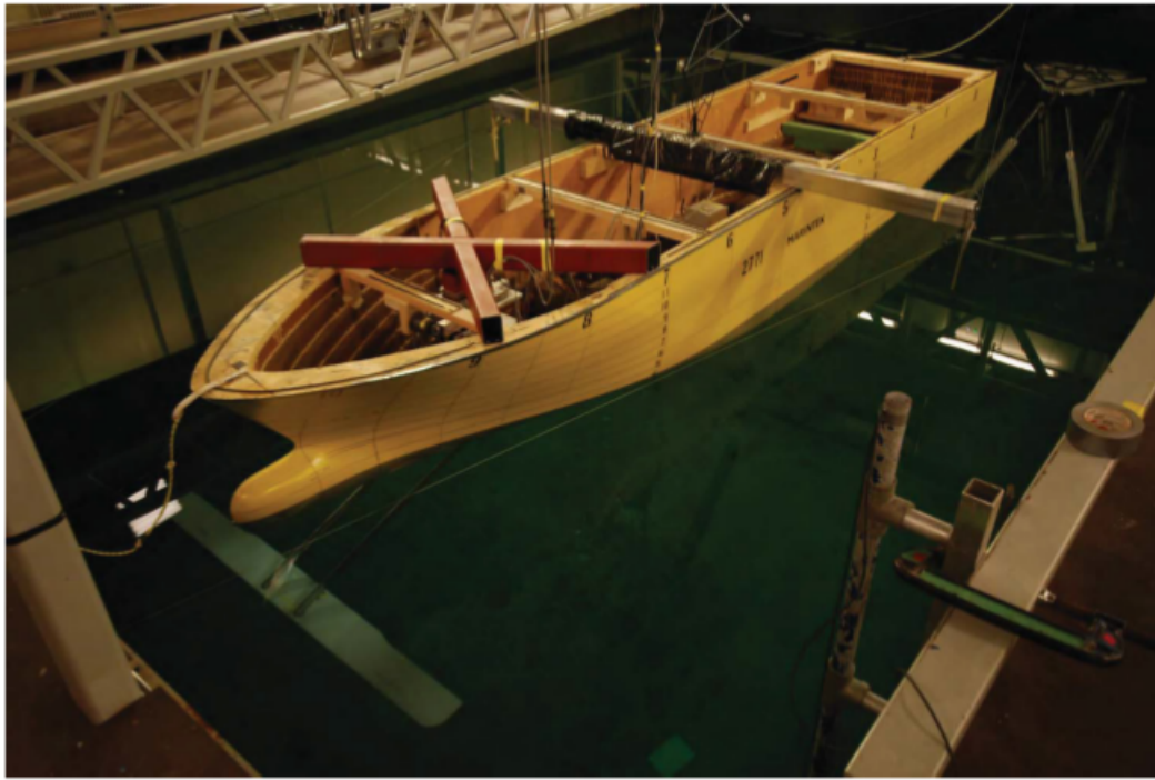
Figure 1.7: Bøckmann (2015) performed experiments with a model equipped with a foil below the hull for motion reduction and thrust production in waves.
