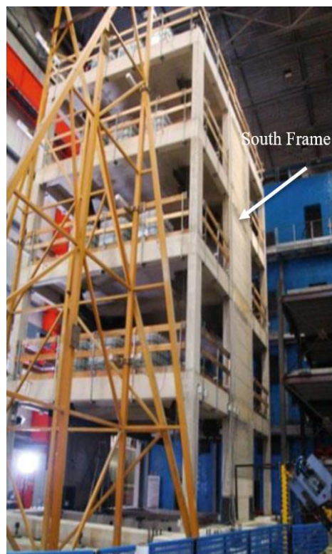
Fig. 8.3 Four-storey RC specimen in the lab. [195]
